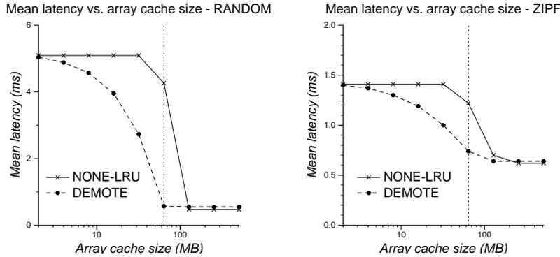
**Figure 6:** Mean READ latency vs. array cache size for the RANDOM and ZIPF workloads. The client cache size was fixed at 64 MB. The 64 MB size is marked with a dotted line.
