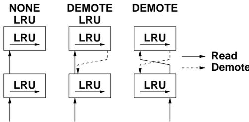
**Figure 1:** Sample cache management schemes. The top and bottom boxes represent the client and array cache replacement queues respectively. The arrow in a box points to the end closest to being discarded.
