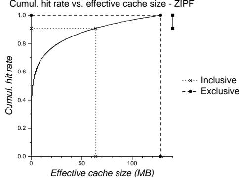
**Figure 2:** Cumulative hit rate vs. effective cache size for a Zipf-like workload, with client and array caches of 64 MB each and a working set size of 128 MB. The marker shows the additional array hit rate achieved with exclusive caching.
