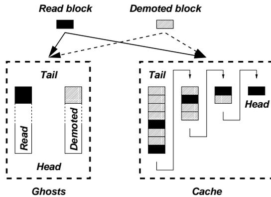
**Figure 8:** Operation of read and demoted ghost caches in conjunction with the array cache. The array inserts the metadata of incoming read (demoted) blocks into the corresponding ghost, and the data into the cache. The cache is divided into segments of either uniform or exponentially-growing size. The array selects the segment into which to insert the incoming read (demoted) block based on the hit count in the corresponding ghost.
