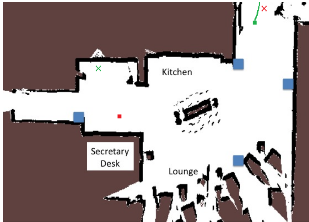
Figure 13.1: A hindrance-sensitive robot path planning problem in our experimental environment containing a person (green square) in the upper right with a previous trajectory (green line) and intended destination (green X) near a doorway, and a robot (red square) near the secretary desk with its intended destination (red X) near the person’s starting location. Hindrances are likely if the person and robot both take the distance-minimizing path to their intended destinations. Laser scanners are denoted with blue boxes.
