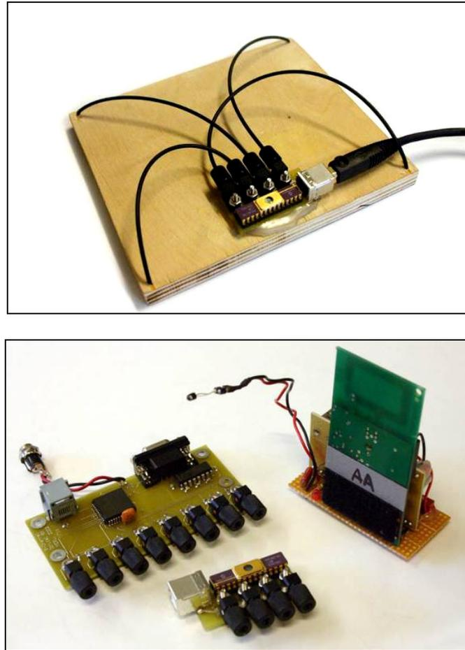
**Figure 4.** Top: A rear view of the instrumented target surface showing the optical fibers and sensor package. Bottom: an 8-channel and 4-channel wired sensor packages and a single wireless RF sensor tag.
