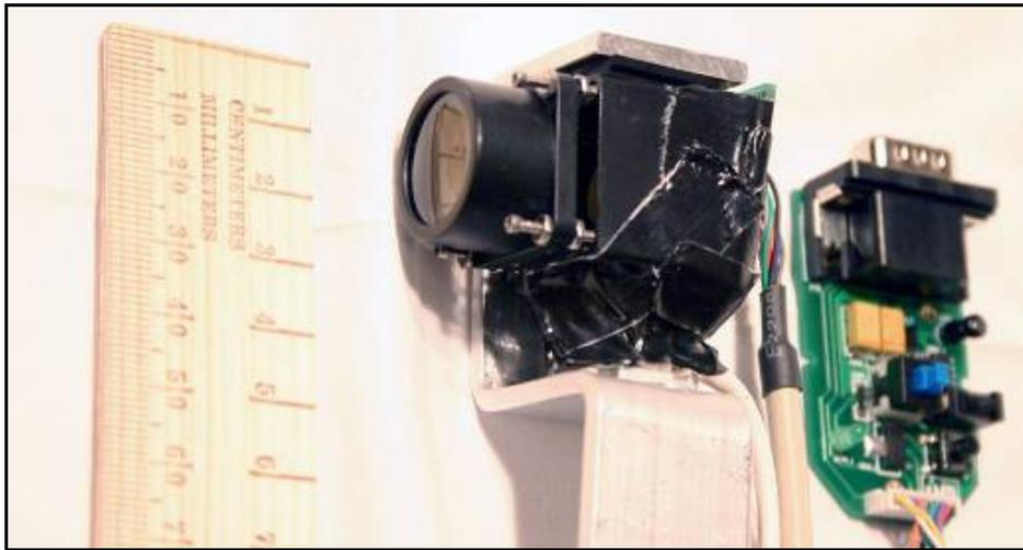
**Figure 9.** Miniature handheld projector prototype.
