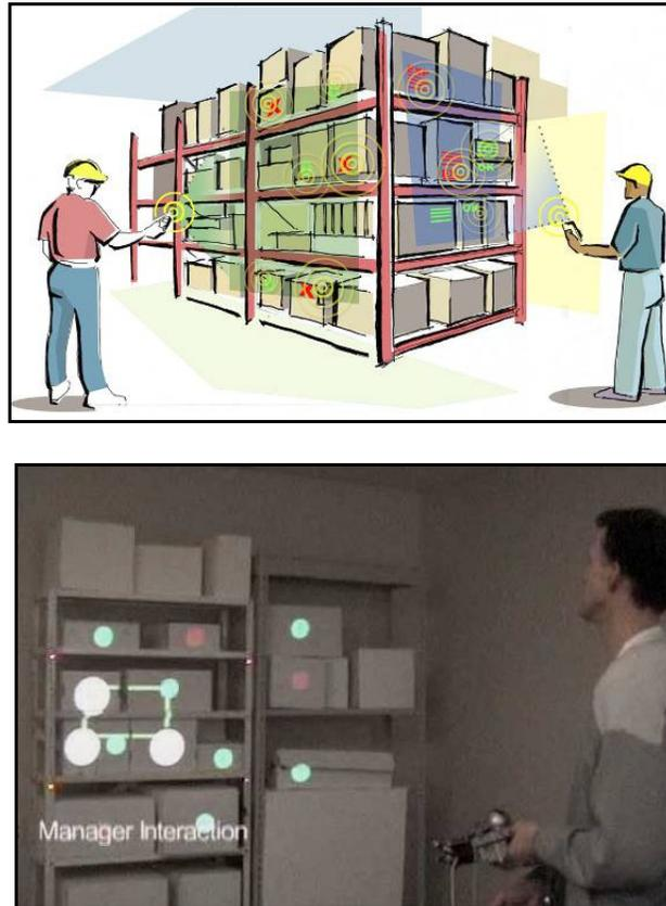
**Figure 8.** Using photosensitive RFID tags and a handheld projector to point, select, and digitally annotate physical objects that have been visually augmented.
