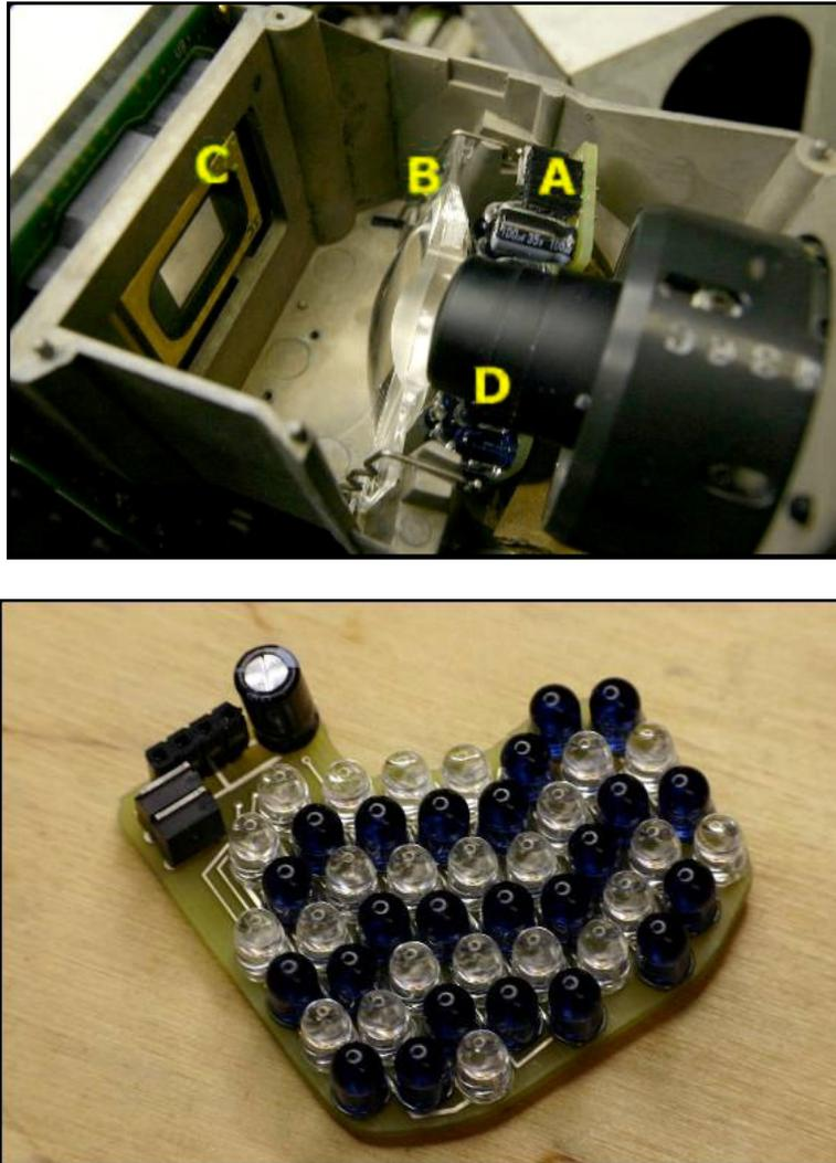
**Figure 17.** Top: Inside the projector A) LED light source B) culminating lens C) DMD device and D) projection lens. Bottom: light source of 24 red (clear) and 24 infrared (dark) LEDs
