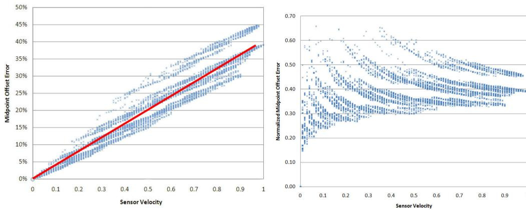
**Figure 28.** Offset encoding error of a sensor moving linearly in a Gray-coded projection area relative to the total pattern width (left) and normalized to the size of the movement (right).
