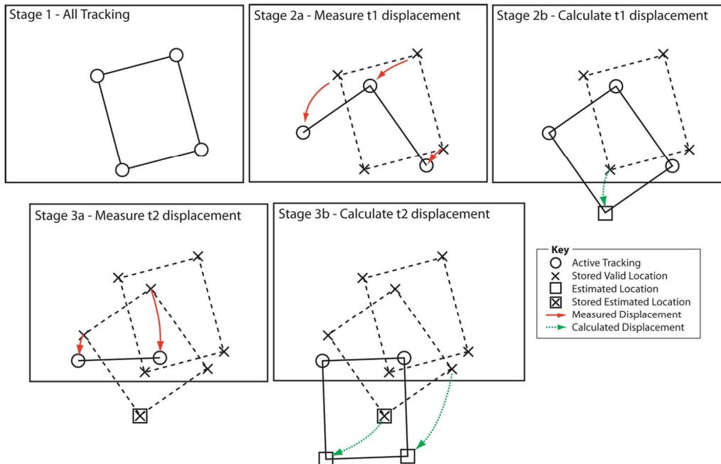
**Figure 12.** Illustration of the sensor location estimation process when dealing with 0, 1, and 2 unavailable sensors.
