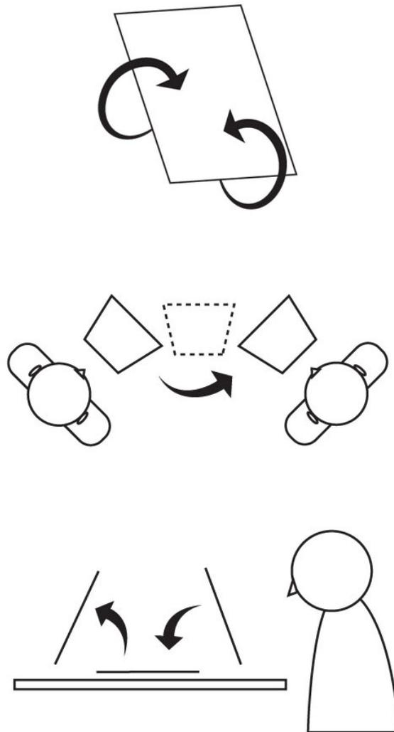
**Figure 23.** Orientation sensitivity behaviors (left to right): double-sided display surfaces can react differently depending on the direction they are flipped, simulated lenticular can change the document view depending on the angle of viewing in a hand-held display, or a tabletop scenario where tilt angle may correspond to different privacy states: *private*, *public*, *excluded*.
