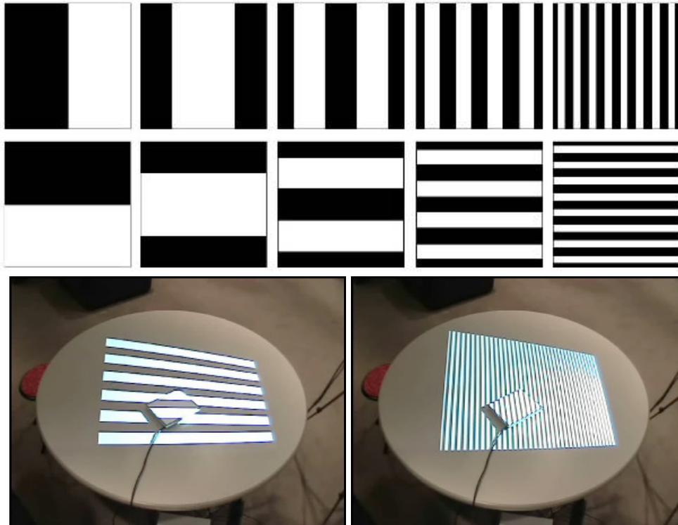
**Figure 1.** This set of horizontal and vertical Gray-coded binary patterns (top) are sequentially projected (bottom) to discover the  $x$  and  $y$  pixel coordinates of each sensor.
