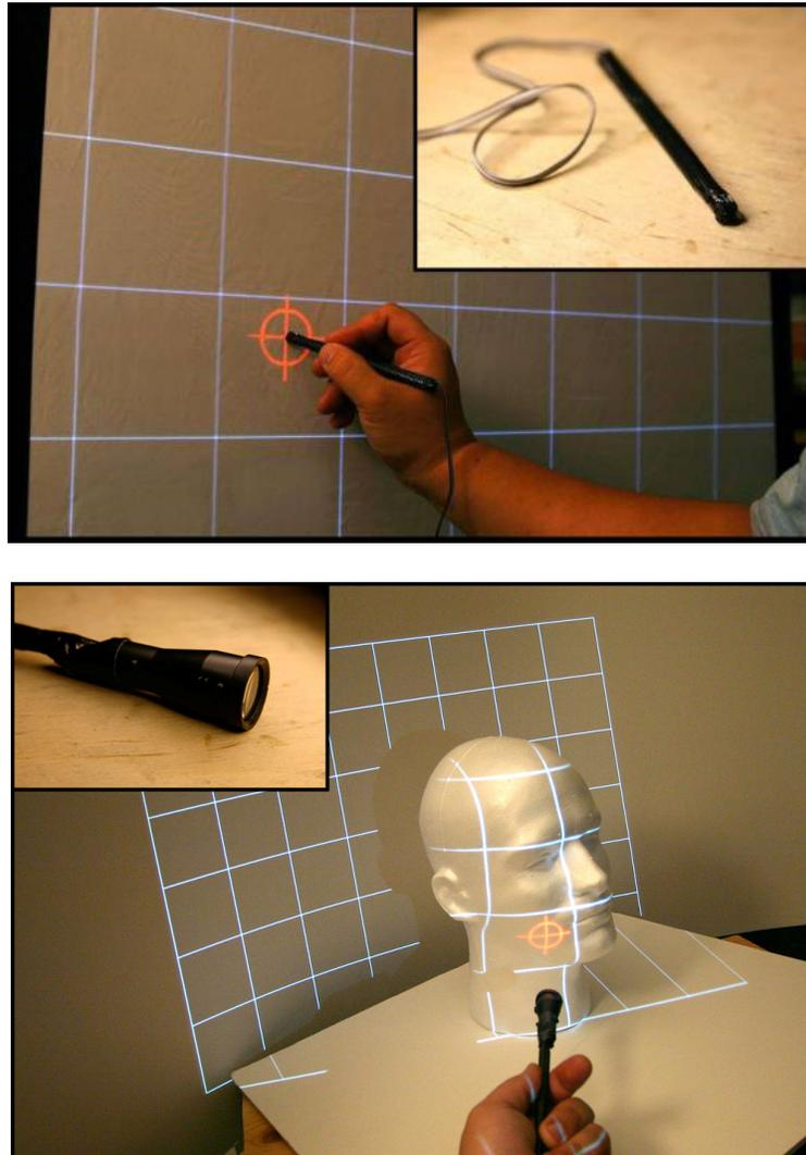
**Figure 19.** Top: A stylus with a light sensing tip (insert) user to interact with a rear-projected display. Bottom: a stylus with a focusing lens mounted on the tip (insert) for distant pointing on non-planar and discontinuous surfaces.
