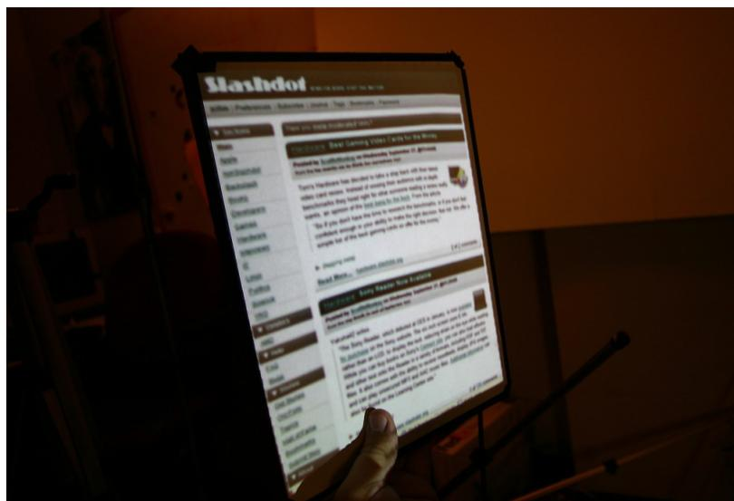
**Figure 18.** Tracking the location of a hand-held surface containing four IR receivers (top) and then projecting visible application content onto that surface to simulate an active display(bottom).
