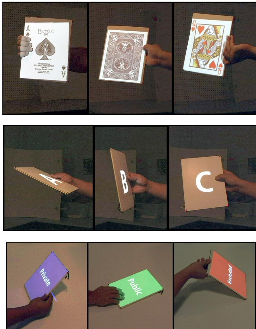
**Figure 24.** Orientation sensitivity prototypes: (top) double-sided flip direction, (middle) vertical and horizontal simulated lenticular in a hand-held surface, and (bottom) a tabletop scenario where tilt correlates to different privacy states.
