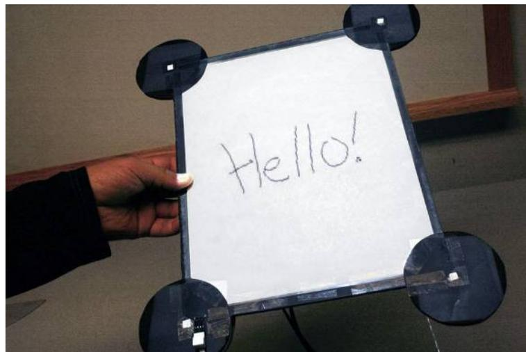
**Figure 11.** A handheld surface containing optical sensors and a touch sensitive surface is tracked using project-based tracking. The location data is then used to project content that matches the surface movements simulating an ultra-lightweight tablet display at low-cost.
