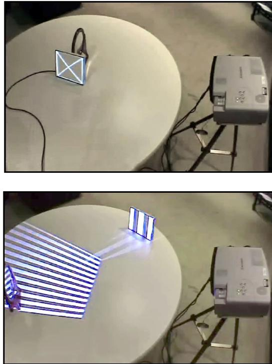
**Figure 3.** Location discovery of sensor continues to work even under very shallow projection angles (top) and when the optical path is folded using a mirror (bottom).
