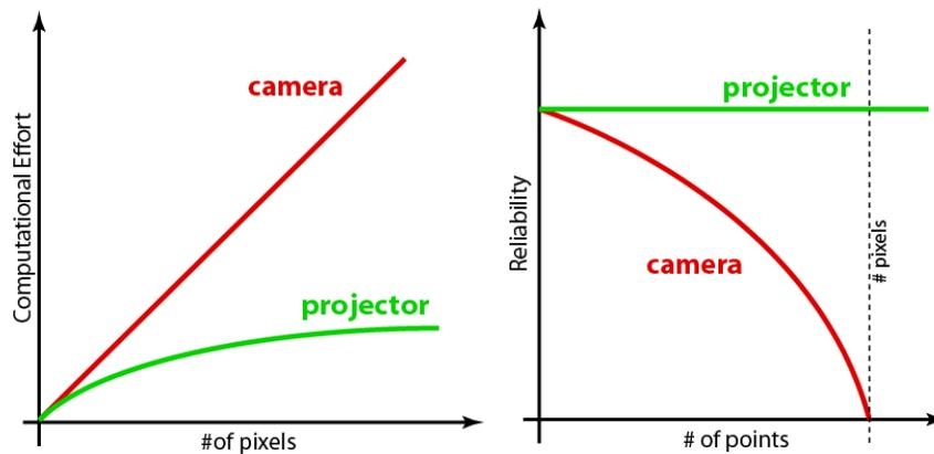
**Figure 26.** Scalability comparisons between camera-based and projector-based tracking for computational effort (left) and multi-point tracking (right).
