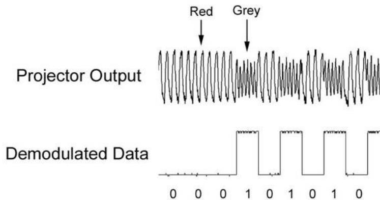
**Figure 10.** Frequency modulated pattern transmission using two colors
