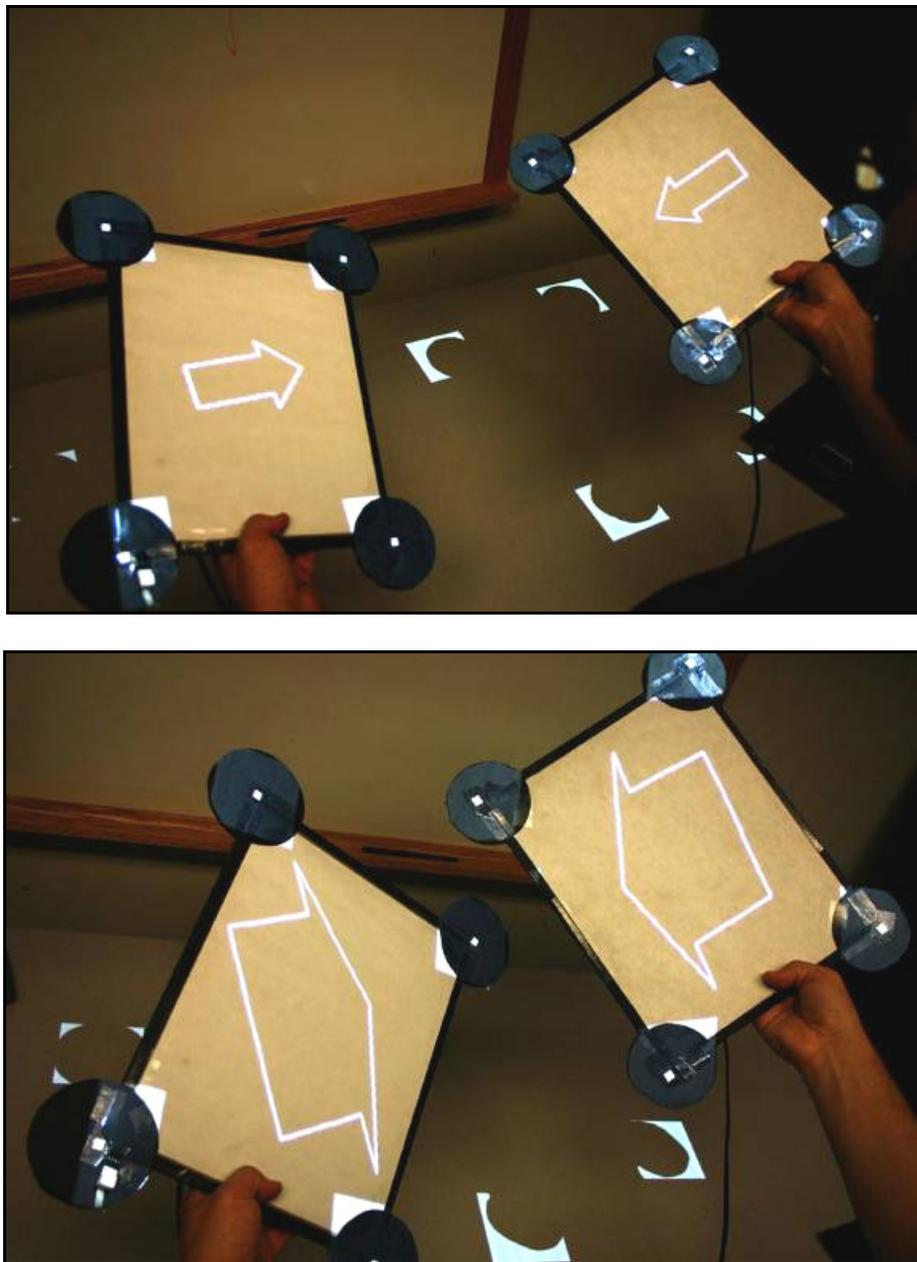
**Figure 14.** Location sensitive multi-display interaction. The projected arrows reflect the direction and distance to the other surface.
