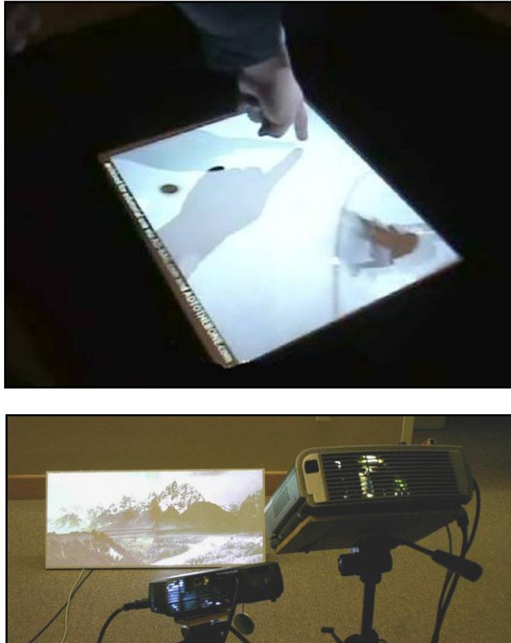
**Figure 5.** Multi-projector applications: image layering (top) and image stitching (bottom)
