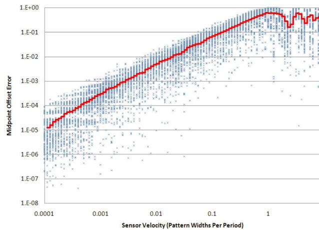
**Figure 29.** Offset encoding error of a sensor moving sinusoidally in a Gray-coded projection area.
