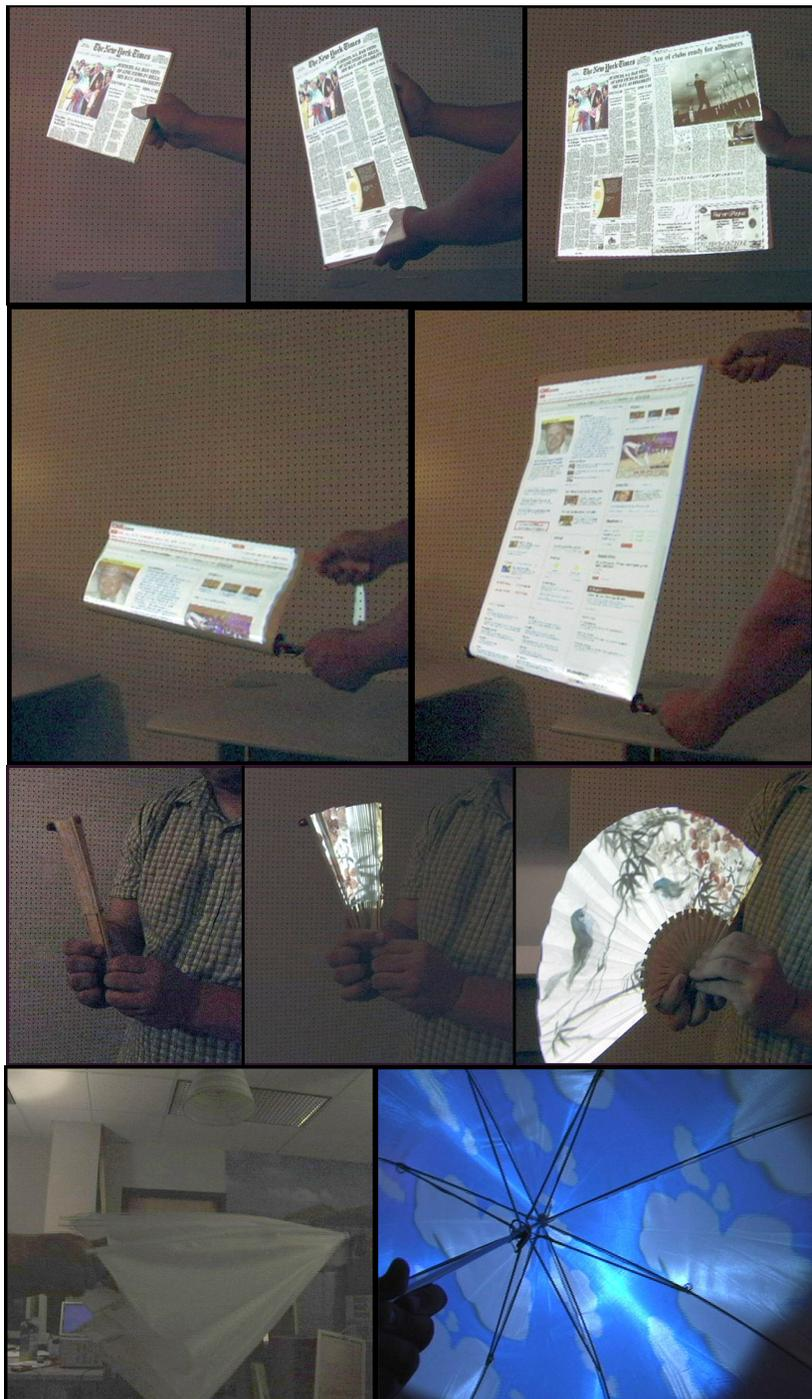
**Figure 22.** Foldable display prototypes at various stages of expansion (top to bottom): newspaper, scroll, fan, and umbrella
