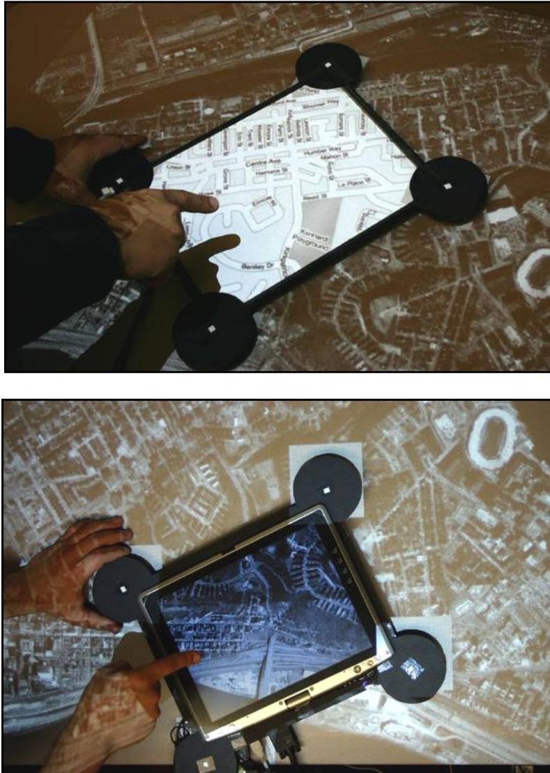
**Figure 13.** Magic Lenses using only a projector (top) and with a high-resolution display (bottom)
