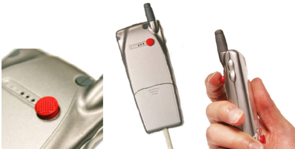
Figure 8.4. The back isometric joystick used by the index finger.
