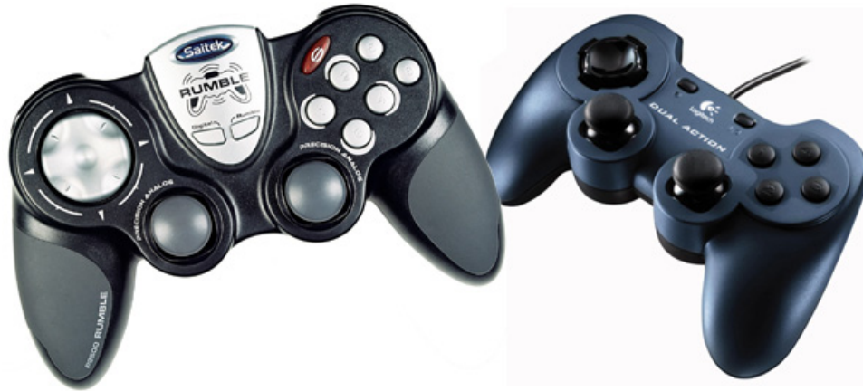
Figure 5.1. The Saitek P2500 and Logitech Dual Action Gamepad, both of which have square areas around their thumb-controlled sticks. If released, both sticks snap to center.
