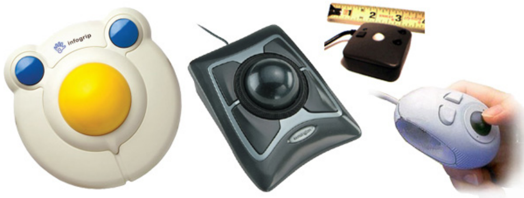
Figure 7.1. Trackballs come in many different sizes making them appropriate as computer access and mobile technologies. From left to right: Infogrip BIGTrack ( http://www.infogrip.com ), Kensington Expert Mouse ( http://www.kensington.com ), Appoint Thumbelina , and Infogrip’s Mini Trackball . Relative image sizes are maintained.
