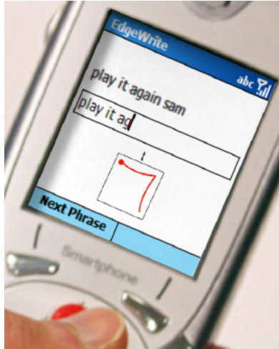
Figure 8.6. Special software on the phone “caught” the recognized characters from the desktop computer and displayed them on the phone’s screen. It also drew stroke traces for Isometric Joystick EdgeWrite.
