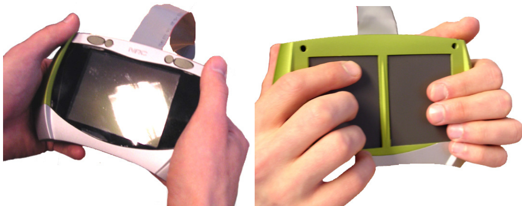
Figure 2.10. Silfverberg et al. 's prototype. In the right image, the left touchpad is used to pan in four directions, and the right touchpad is used to zoom. Used with permission.
