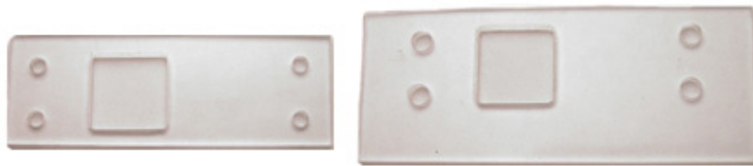
Figure 4.5. Two plastic templates, each with a 1.69 cm 2 hole.
