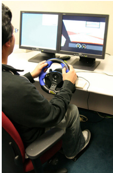
Figure 10.2. The experimental setup with the STISIM driving simulator. The list of street names and input techniques are shown on the left monitor as peripheral heads-up display.
