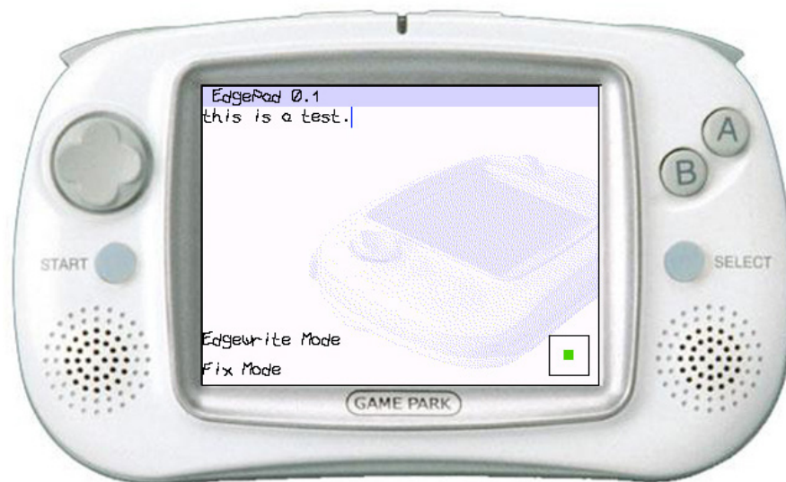
Figure 10.6. The GP32 device and the EdgePad text entry utility. Used with permission.
