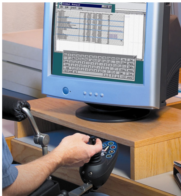
Figure 6.1. The Mouse Driver system from Switch-It, Inc. enables a wheelchair joystick to control a mouse cursor on a desktop PC. Unfortunately, text entry reduces to pointing with an on-screen keyboard. Image from http://www.switchit-inc.com .
