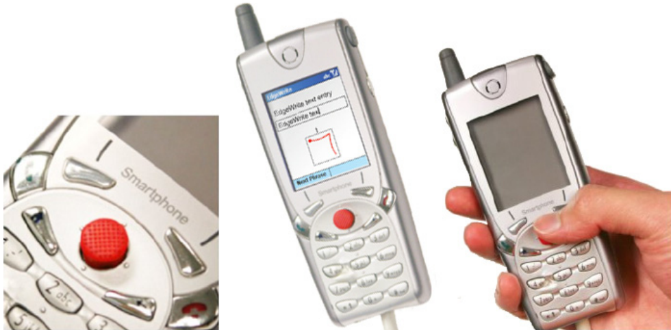
Figure 8.3. The front isometric joystick used by the thumb.
