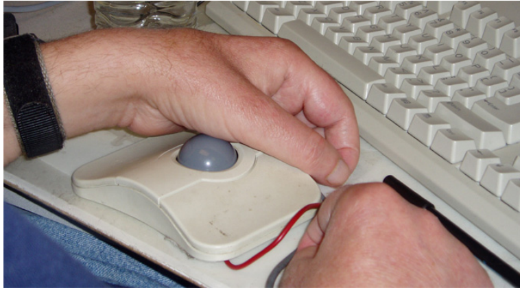
Figure 7.13. Jim’s favorite trackball is the Stingray because he can press its wide left button with the palm of his left hand while his left thumb rolls the ball to drag.
