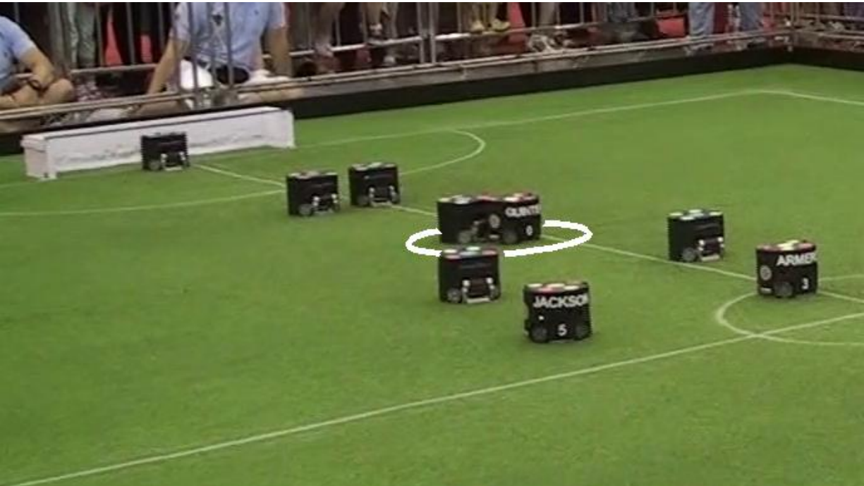
Figure 6.10: An example of the visualization shown when the ball is in the process of becoming stuck during play. The ball is stuck between the two robots in the white circle.
