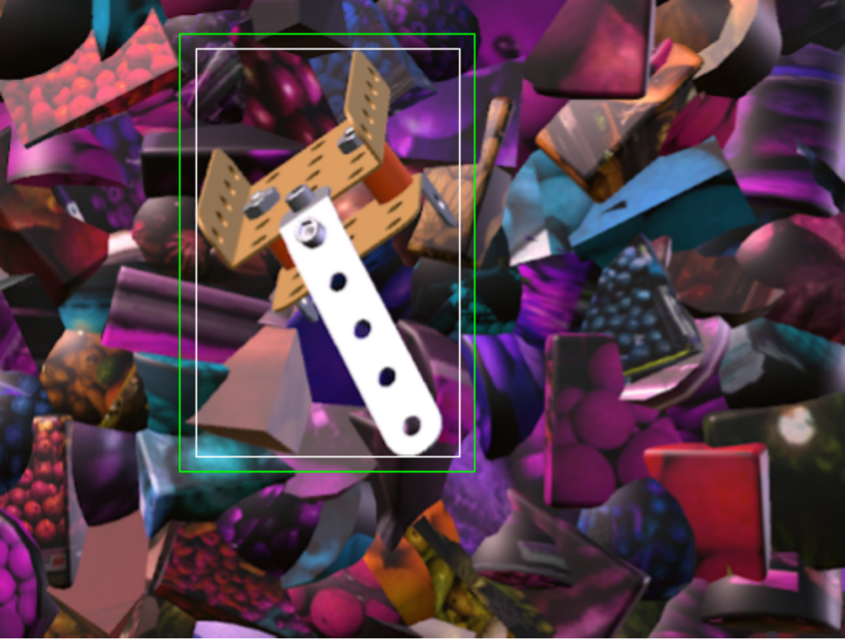
Figure 4.4: Bounding boxes with and without padding. The white bounding box has no padding. The Unity perception package uses bounding boxes without padding. The green bounding box has padding. Our dataset uses bounding boxes with padding.
