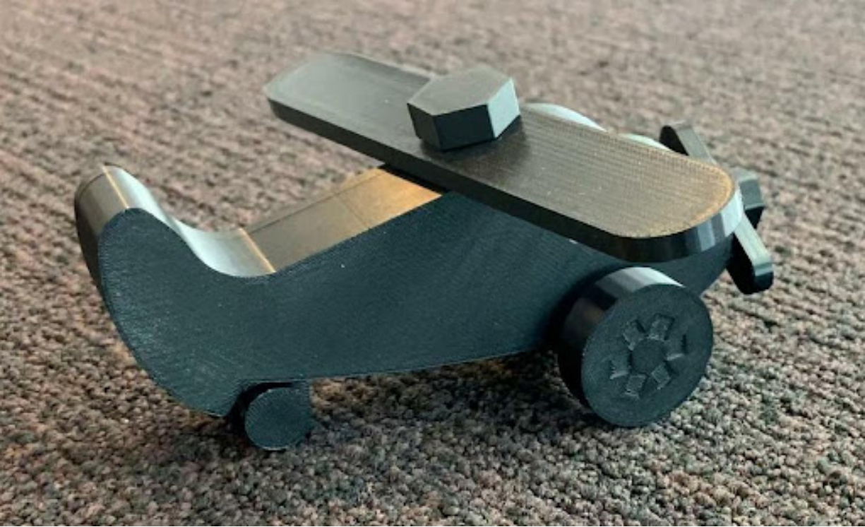
Figure 4.9: The fully assembled model plane kit. All parts are 3D printed plastic.
