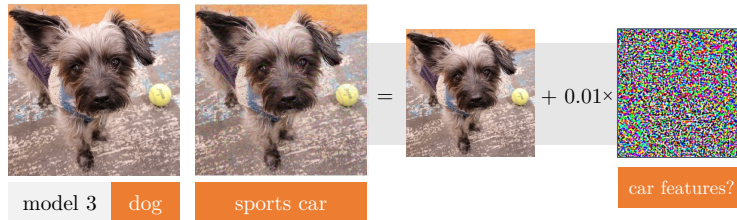
Figure 1.2: Prediction of a model on an image of a dog (left) and a perturbed image (right) derived by adding barely-perceptible noise-like features to the original image. We see that the model makes the correct prediction on the original image, but incorrectly predicts “sports car” on the perturbed image rather than “dog.” This discrepancy suggests that the model perceives the noise-like features as indicators of sports cars.
