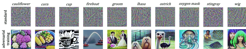
Figure 8.10: Example reconstructions from publicly available pre-trained ResNet50 ImageNet models for both standard and adversarial training. The column labels indicate the ImageNet class that was targeted for reconstruction. (top) standard model available from Torchvision. 2 (bottom) adversarially trained model available from MadryLab. 3
