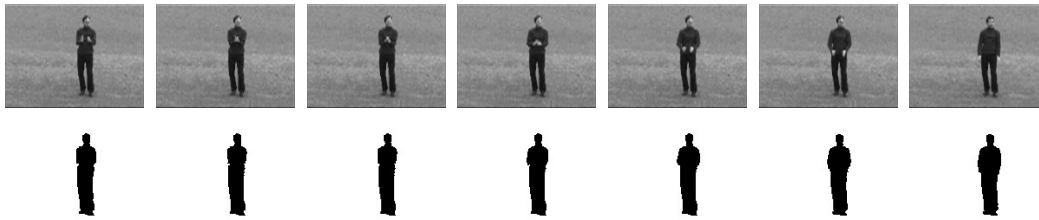
FIGURE 4.13. Notice how the silhouette stays constant during this part of the hand-clapping event. More generally, a fundamental limitation of such shape features is that they cannot represent motion inside the silhouette.
