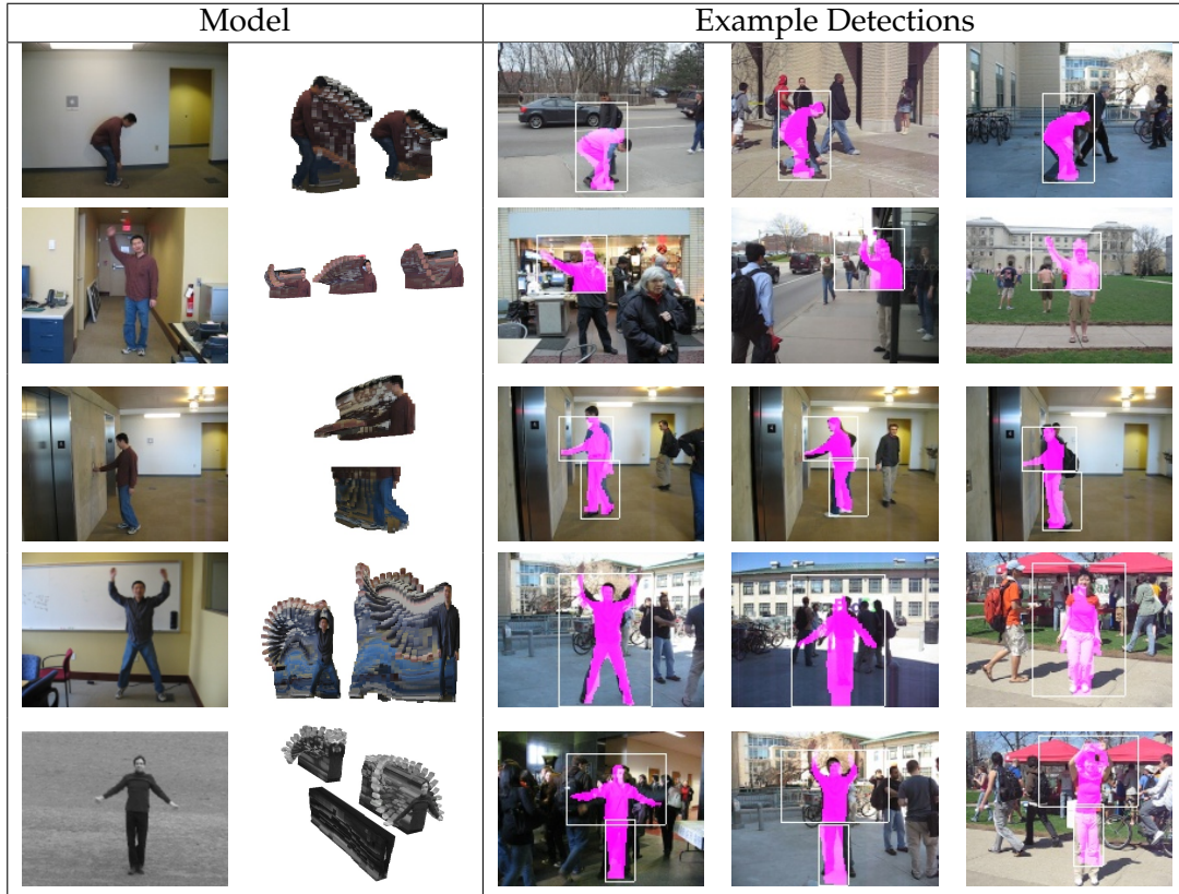
FIGURE 5.3. Examples of event detection in crowded video. Training sequences and event models are shown on the left. Detections in challenging test sequences are shown on the right. The action mask from the appropriate time in the event model is overlaid on the test sequence, and a bounding box drawn around each part.
