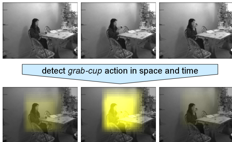
FIGURE 3.1. An example of our detector recognizing the grab-cup action. Note that the detection volume (shown highlighted) is localized both in space and time.
