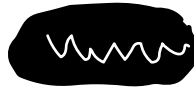
Figure 3-7. Buttons are drawn in reverse video when the mouse button is held down over them. The feedback is removed when the mouse is released.
