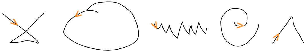
Figure 1-14. Editing gestures for delete, group, ungroup, change inference, and text editing. The arrows indicate a recommended direction to draw these gestures for best recognition performance.
