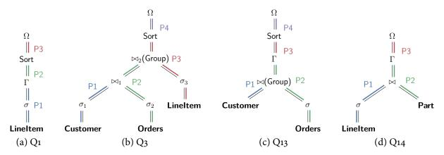
**Figure 3.6: TPC-H Query Plans with Pipelines** – The high-level query plan for the subset of the TPC-H queries that we evaluate in our experiments, and do deep-dive analysis on. Each plan is annotated with their pipelines [108].
