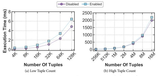
**Figure 5.7: Compression with Increasing Tuple Counts** – Measuring hash join performance with PCG compression when varying the size of the materialized hash table but with a fixed compression factor and tuple size.
