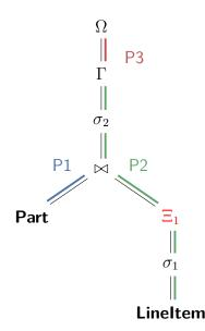
**Figure 3.2: Example Query Plan Using ROF** – The physical query plan for TPC-H Q19 using our relaxed operator fusion model.
