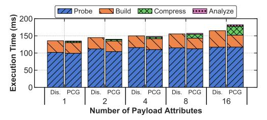
**Figure 5.6: Compression with Varying Tuple Size** – A breakdown of the time to perform a hash join with and without PCG compression when varying the number of non-key attributes in the build-side tuple.
