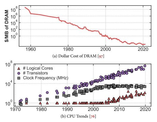
**Figure 1.1: Modern Hardware Trends** – From (a) we observe that DRAM manufacturing costs have consistently fallen from the early 1960s. In (b) we observe that although Moore's law [106] remains correct even in today's ecosystems [45, 54], clock frequencies have plateaued due to physical limitations in the CPUs ability to dissipate heat [32]. To compensate and continue to offer improved performance, CPU manufacturers rely on increasing core counts.
