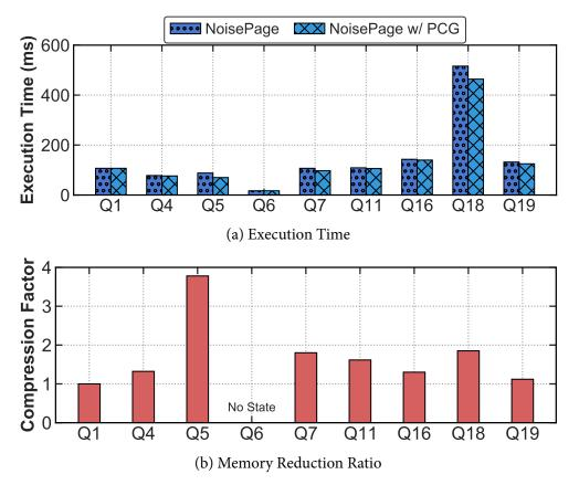
**Figure 5.13: TPC-H Performance** – Evaluation of a selection of TPC-H queries with and without memory compression enabled using PCG. (a) and (b) show the query performance and memory reduction ratio, respectively.
