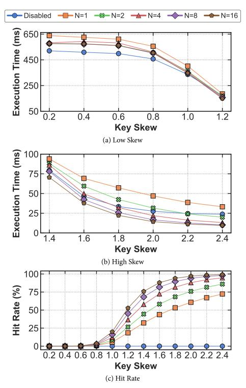
**Figure 5.12:** Varying Join Key Skew – Performance of PCG's join key specialization when increasing skew in the join keys. (a) and (b) plot the total execution time when the skew is low and high, respectively; (c) shows the percentage of hash table probes that hit a heavy-hitter branch.
