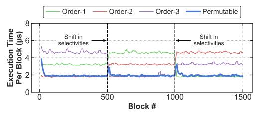
**Figure 4.6: Performance Over Time** – Execution time of three static filter orderings and the PCQ filter as we perform a sequential scan over a table.
