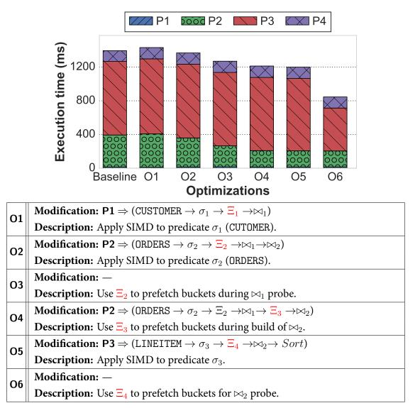
**Figure 3.9: Q3 Case Study** – The breakdown of the ROF optimizations applied to TPC-H Q3 query plan shown in Figure 3.6b.
