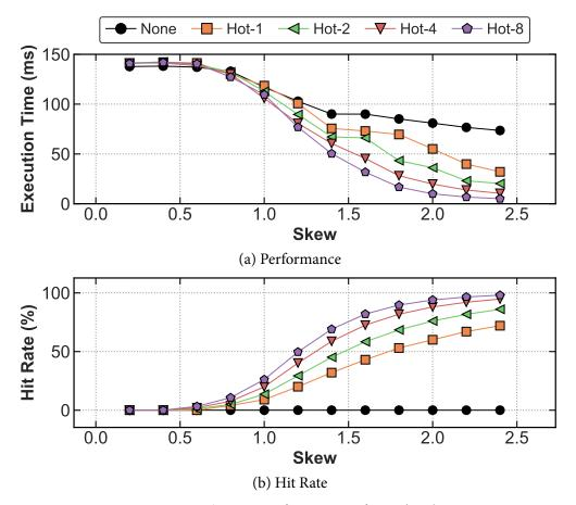
**Figure 4.10: Varying Aggregation Skew** – Performance of PCQ's adaptive aggregation when increasing skew in aggregate keys with a fixed number of keys. (a) shows the total execution time to perform the aggregation. (b) shows the percentage of input tuples that hit a heavy-hitter branch.
