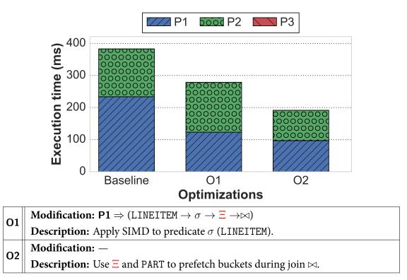
**Figure 3.11: Q14 Case Study** – The breakdown of the ROF optimizations applied to TPC-H Q14 query plan shown in Figure 3.6d.
