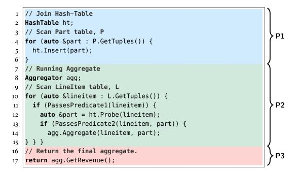
**Figure 2.2: Query Compilation Example** – The generated code for TPC-H Q19 (Figure 2.1) using a tuple-at-a-time processing model.
