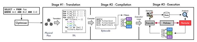
**Figure 4.2: System Overview** – The DBMS translates the SQL query into a DSL that contains indirection layers to enable permutability. Next, the system compiles the DSL into a compact bytecode representation. Lastly, an interpreter executes the bytecode. During execution, the DBMS collects statistics for each predicate, analyzes this information, and permutes the ordering to improve performance.
