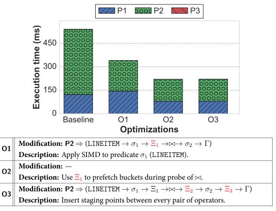
**Figure 3.12: Q19 Case Study** – The breakdown of the ROF optimizations applied to TPC-H Q19 query plan shown in Figure 2.1b.
