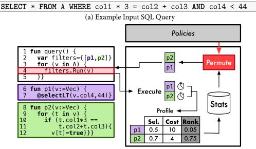
(b) Generated Code and Execution of Permutable Filter
