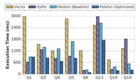
**Figure 3.16: System Comparison** – Performance evaluation of the TPC-H benchmark in Vector, HyPer, and Peloton with and without our ROF model.
