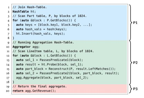
**Figure 2.3: Vectorization Example** – An execution plan for TPC-H Q19 from Figure 2.1 that uses the vectorized processing model.
