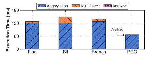
**Figure 5.1: Knowing the Future** – Deferring code generation enables dynamically specializing instructions to data the query has actually processed.
