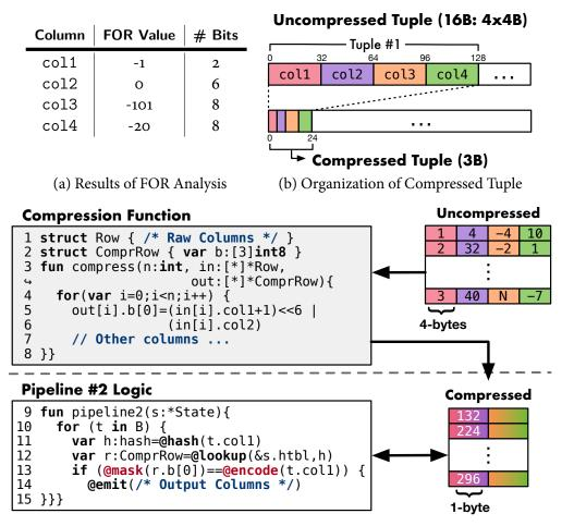
(c) Generated Code With Execution of Compression and Probe
