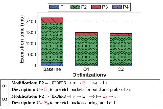
**Figure 3.10: Q13 Case Study** – The breakdown of the ROF optimizations applied to TPC-H Q13 query plan shown in Figure 3.6c.
