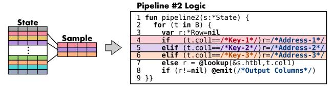
**Figure 5.5:** Specializing Join Probing Logic – If the DBMS detects join key skew, it samples the input to collect a representative set of "hot" keys, probes the hash table once before generating the probe logic, then generates explicit checks for each key, embedding the address of the result if successful.
