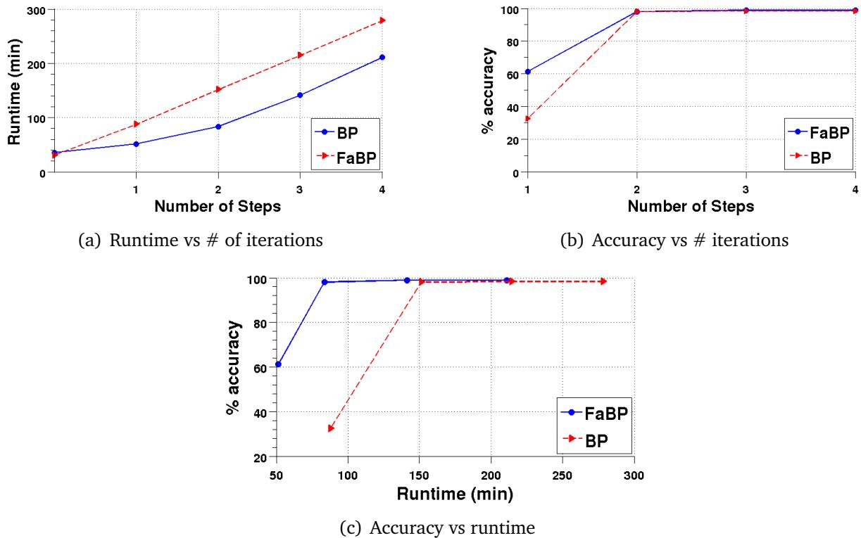
**Figure 4.7: Performance on the YahooWeb graph (best viewed in color):** FABP wins on speed and wins/ties on accuracy. In (c), each of the method contains 4 points which correspond to the number of steps from 1 to 4. Notice that FABP achieves the maximum accuracy after 84 minutes, while BP achieves the same accuracy after 151 minutes.
