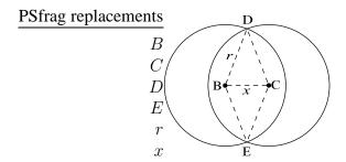
The figure above indicates the parameters to be used in our calculation. B and C denote two communicating sensor nodes. r is the communications range of each sensor node. We assume that each node has the same range for receiving and transmitting. x is the distance between two nodes.
