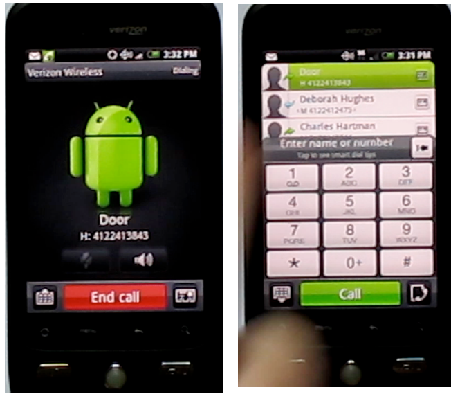
Figure 1.1: On some cellular phones the “End Call” button transforms into a “Call” button when the other party hangs up. A user attempting to use the button may reestablish a call with the other party by mistake.
