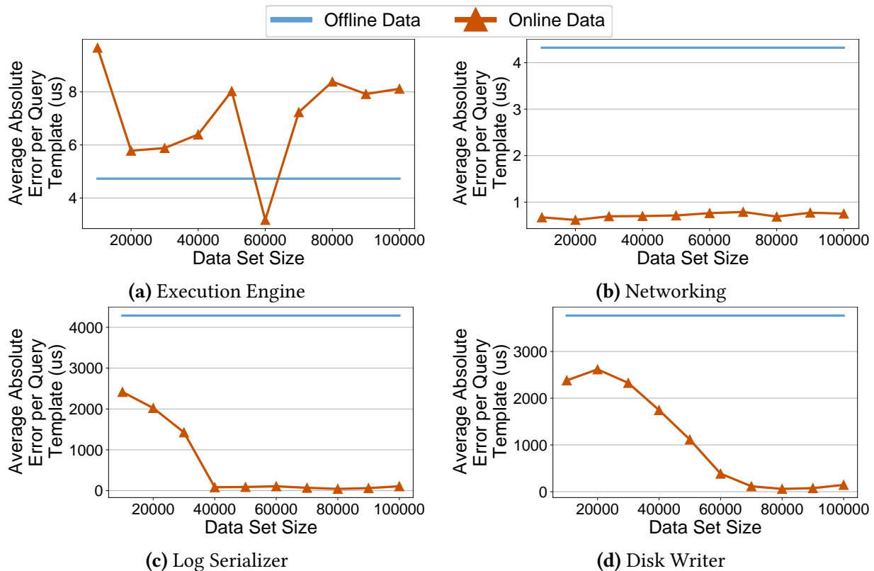
Figure 3.9: Model Convergence (TPC-C) – Comparing prediction error of baseline OU models trained with offline runner data against models trained with increasing size online TPC-C data.
