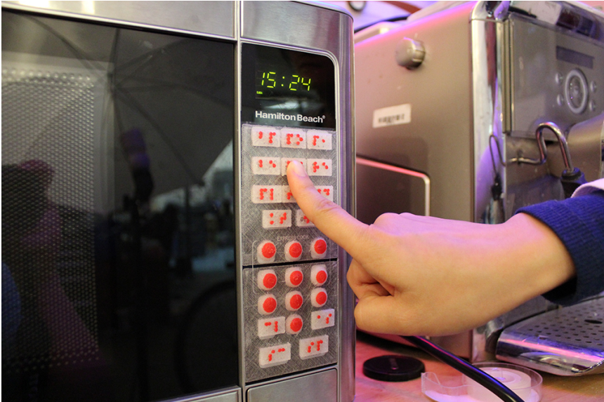
Figure 1.2: Facade is a crowdsourced fabrication pipeline that enables blind people to make flat physical interfaces accessible by independently producing a 3D-printed overlay of tactile buttons.
