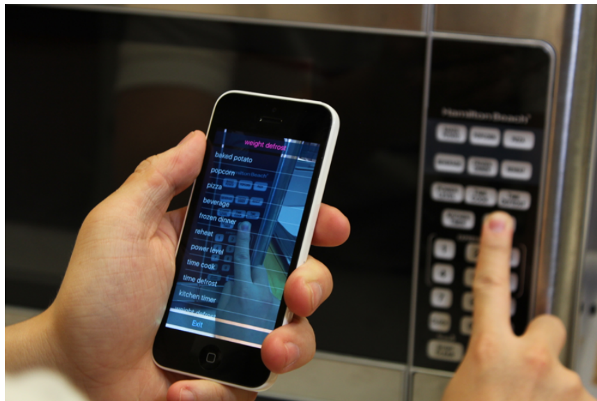
Figure 1.1: VizLens is a screen reader to help blind people access static physical interfaces.
