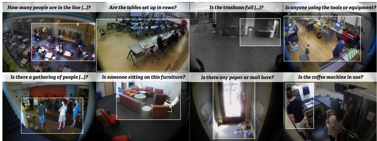
Figure 1.4: Eight example sensors created by our participants using Zensors++, with regions of interest highlighted on the full camera image. Many sensors directly complemented and augmented people’s existing work practices.
