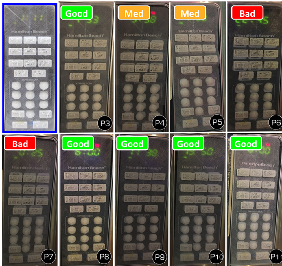
Figure 5.6: Examples of the attached overlay performed by the participants. For P4 and P5, slight offset did not affect using the appliance. An exact alignment is shown in the top left corner.
