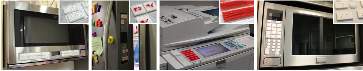
Figure 5.1: Facade is a crowdsourced fabrication pipeline that enables blind people to make flat physical interfaces accessible by independently producing a 3D-printed overlay of tactile buttons. From left to right, we demonstrate example applications including microwave, refrigerator door, copier, and another microwave. Insets shows close views of individual embossed buttons.
