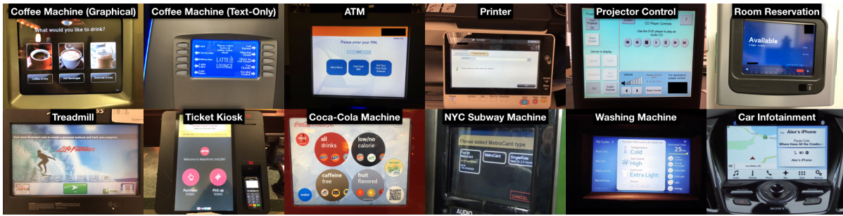
Figure 6.6: We evaluated how well StateLens reconstructs state diagrams from point-of-view usage videos across a wide range of interfaces, including an ATM, coffee machine (both graphical and text only), printer, projector control, room reservation panel, treadmill, ticket kiosk, Coca-Cola machine, subway ticket machine, washer, and car infotainment system.
