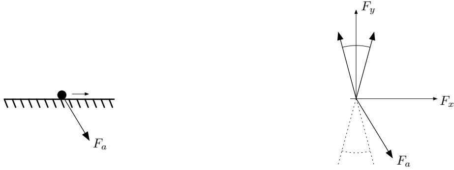
Figure 86: Since the applied force F_a lies outside the negated friction cone, the particle accelerates toward the right.
