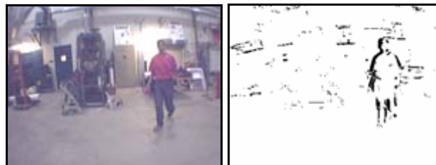
Figure 7. Original Frame (left) & Image Subtraction (right)
