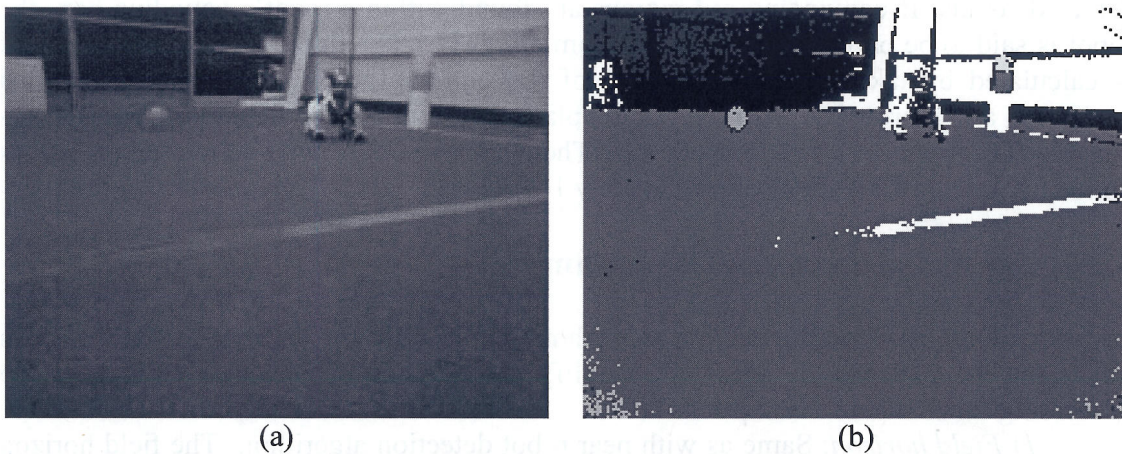
Figure 3.6: (a) Grayscale image of robot on playing field. (b) Color segmented image of the same scene.
