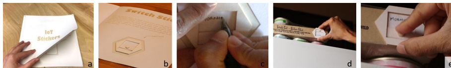
Figure 5: This chapter introduces the IoT Codex: a book of inexpensive, battery-free sensors and interaction patterns to support linking everyday objects to software and web services using stickers. To use, a sticker is first found in the book (a-b), customized (c), peeled from the book and attached to a desired everyday object (d), and then invoked using its kinetic mechanism (e). Stickers can be customized during setup and composed with others to create more expressive applications using the composition space in the book’s pages.
