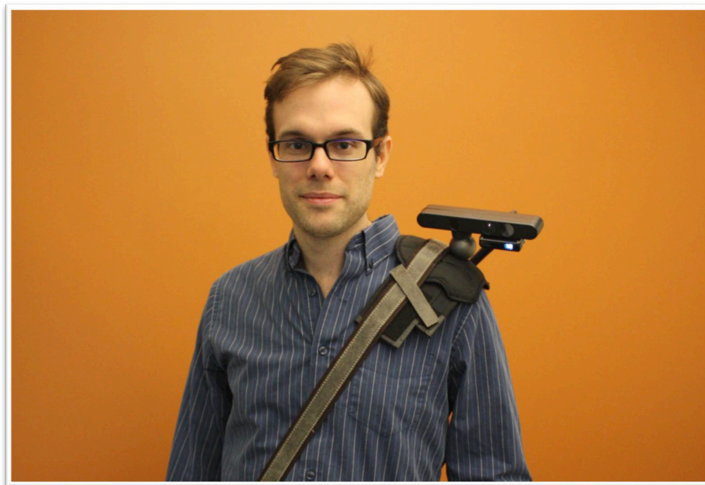
Fig. 4.2 A later OmniTouch prototype that attached to the strap of a bag.
