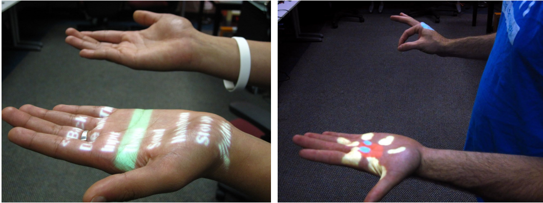
Fig. 6.7 Left: Hierarchical menu navigation on the hand. Right: demonstration tattoo painting application.
