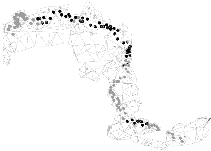
FIGURE 4.7: NPC Plan with SNEAK player, using weighted A* with shortest path heuristic and \epsilon = 100 . The darker dots indicate the player is sneaking.
