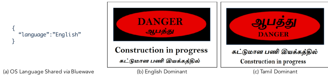
Figure 56. Self-translating sign demonstration. Users share their device’s operating system language via Bluewave (a), and signs can automatically adjust their contents based on the number of nearby users that speak each language (b-c).
