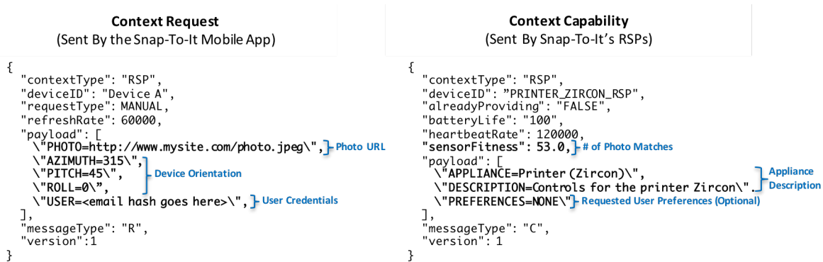
Figure 30. Example Snap-To-It context request (left) and context capability messages (right).
