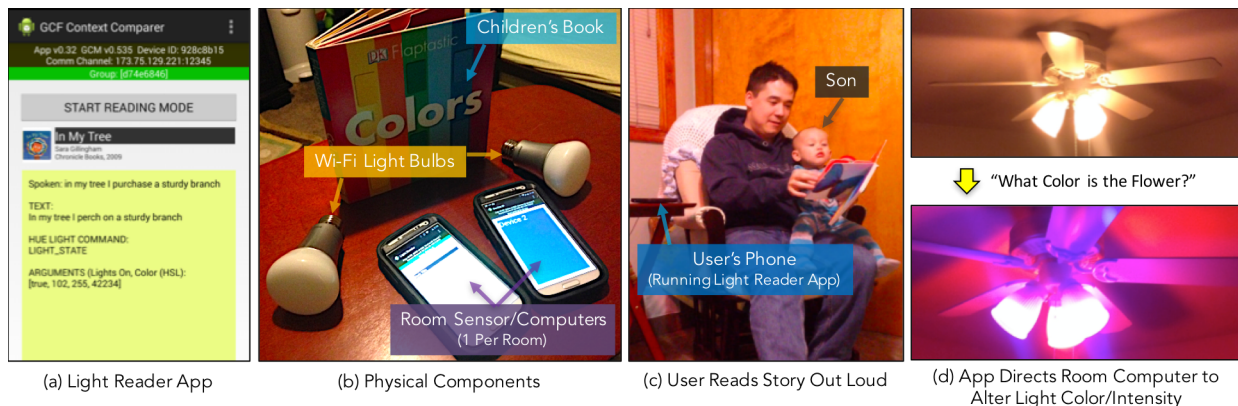
Figure 22. Light Reader system. We created a custom mobile phone application (a) that interfaces with a series of Wi-Fi connected light bulbs and mobile sensors deployed throughout a house (b). When the user reads a book out loud (c), the app uses Didja to form an opportunistic group with the devices in his room. The app then modifies the color and intensity of the lights to match the contents of the story (d).
