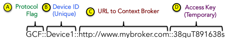
Figure 50. A sample Bluewave device name, containing a fixed length flag (A), the device's unique identifier (B), a URL to the device's context broker (C), and a temporary access key (D).
