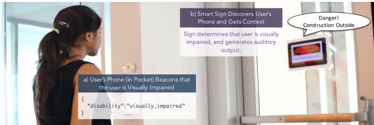
Figure 57. Smart sign demonstration. Users share their disability using Bluewave (a), and smart signs can modify the way they output their contents (b).
