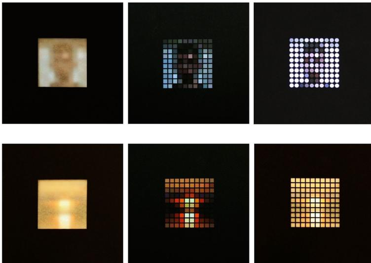
Ultra-low Resolution displays, 10x10 variations displaying an image of a face and a sunset over water. Different forms of light diffusion and tangible grid overlays are employed.
