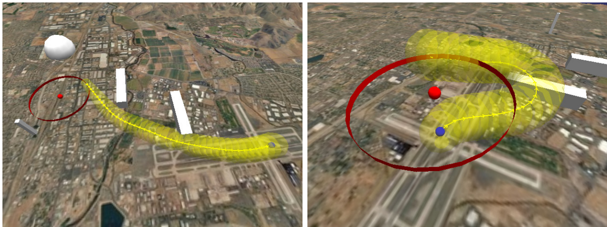
Figure 4.16: Two examples of the fly-to-orbit capability of the UAV planner.
