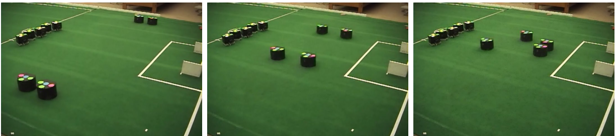
Figure 5.12: A sequence captured while running DSS with four CMDragons robots. All agents completed their 2.8m traversal within 3.1 seconds.
