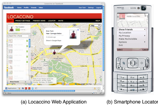
Figure 1: The Locaccino web application (on the left) and the mobile locator installed on a Nokia N95 phone (on the right). The web application is embedded within Facebook, and allows to request friends’ locations, set up privacy settings, and receive privacy-related information. The phone locator reports the user’s location and enables the user to request their friends’ locations.
