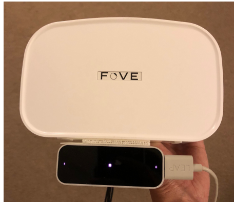
Figure 7.2: Leap Motion was attached underneath the FOVE headset.
