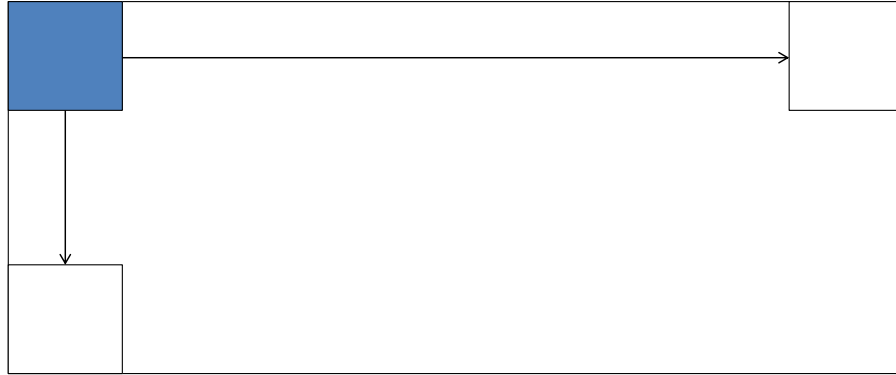
Figure 4.1: A 2D tiled data layout. 2D blocks of data are stored contiguously, allowing efficient traversal along any dimension.
