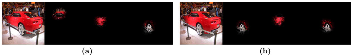
Figure 5.5: (a) Comparative explanation of classes “sports car” and “convertible” taken from the top-three most influential units at the conv4_1 layer (VGG16 [121]). (b) Explanation computed using the quantity of interest corresponding to “sports car” on the same instance used in (a) .
