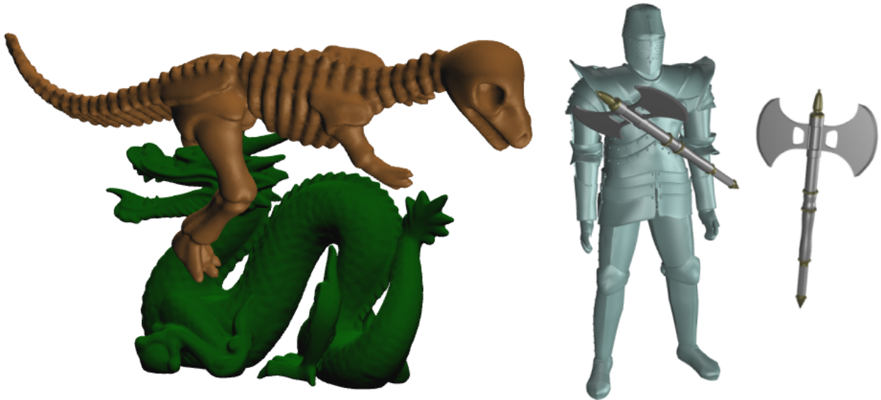
Figure 1.3: Distributed contact: Left: Deformable dragon (deformable pointshell) in contact with a deformable dinosaur (deformable distance field). Right: haptic gaming: attacking the detailed rigid knight with a rigid axe.
