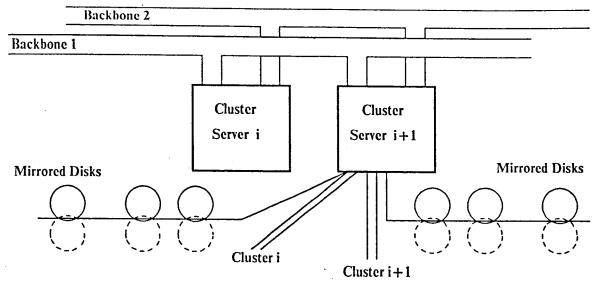
Figure 2: Connections when Cluster Server i is Down
