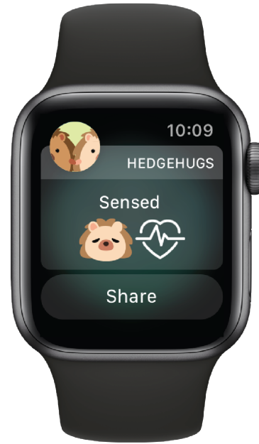
(b) Opening the notification shows an emoji representing the current sensed state (pictured: sad).
