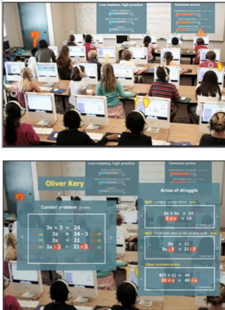
Figure 4-4. Design mock-ups based on findings from low- to mid-fidelity prototyping sessions (from Holstein, Hong, et al., 2018). Top: Teacher’s default view of the class. Each student has an indicator display floating above their head, and class-level analytics displays are positioned at the front of the class. Bottom: “Deep-dive” screens shown if a teacher ‘clicks’ on an indicator. Note: student names shown in this figure are fabricated.
