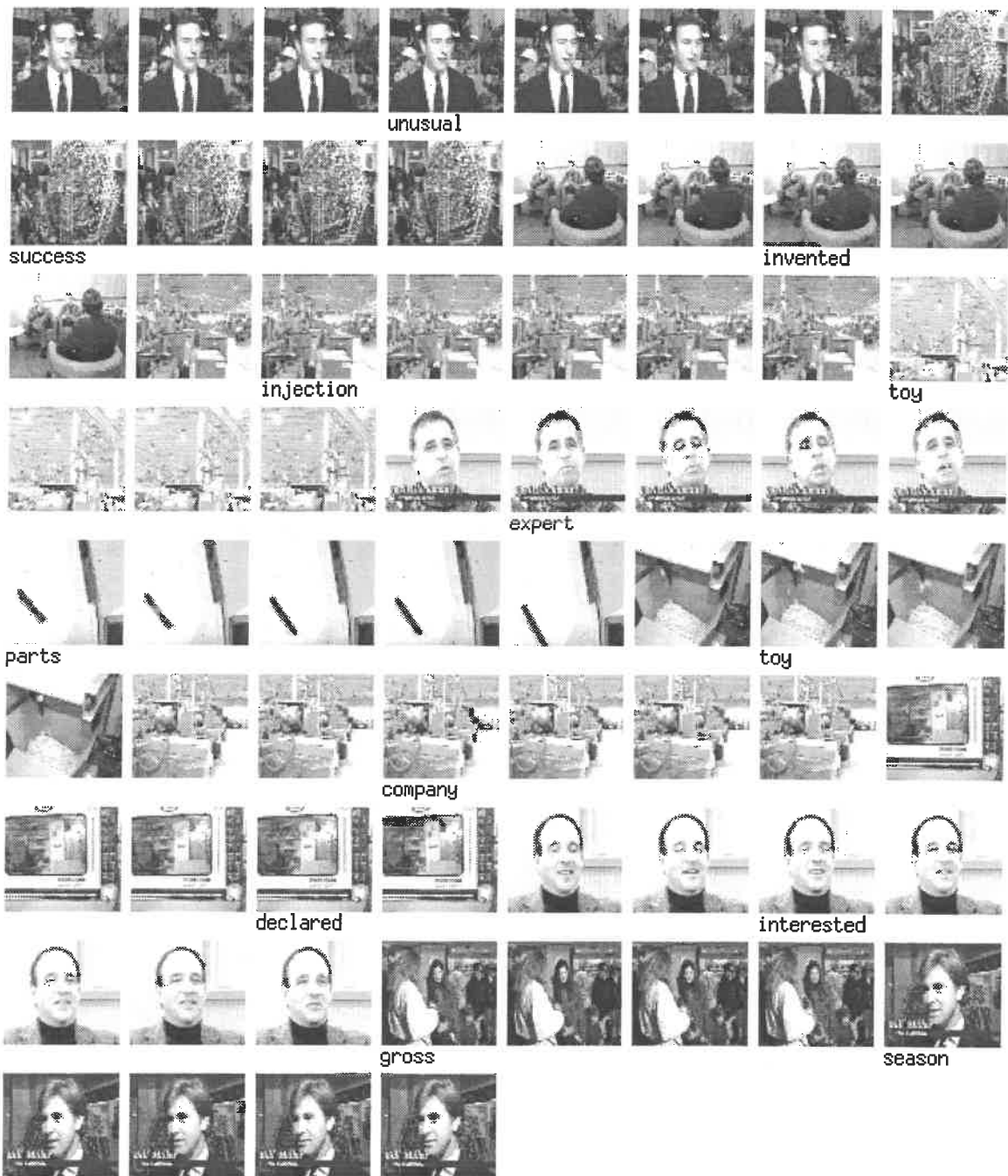
Figure 13b: Skim video frames and audio keywords for the test set, “K’nex Toy”. The word “toy” appears often in this segment and thus has a high TF-IDF weight. Frames with faces and captions have the highest priority. Frames are displayed at 6.0 fps. The length of this skim is 11.33 seconds with the original segment consisting of 61 seconds.
