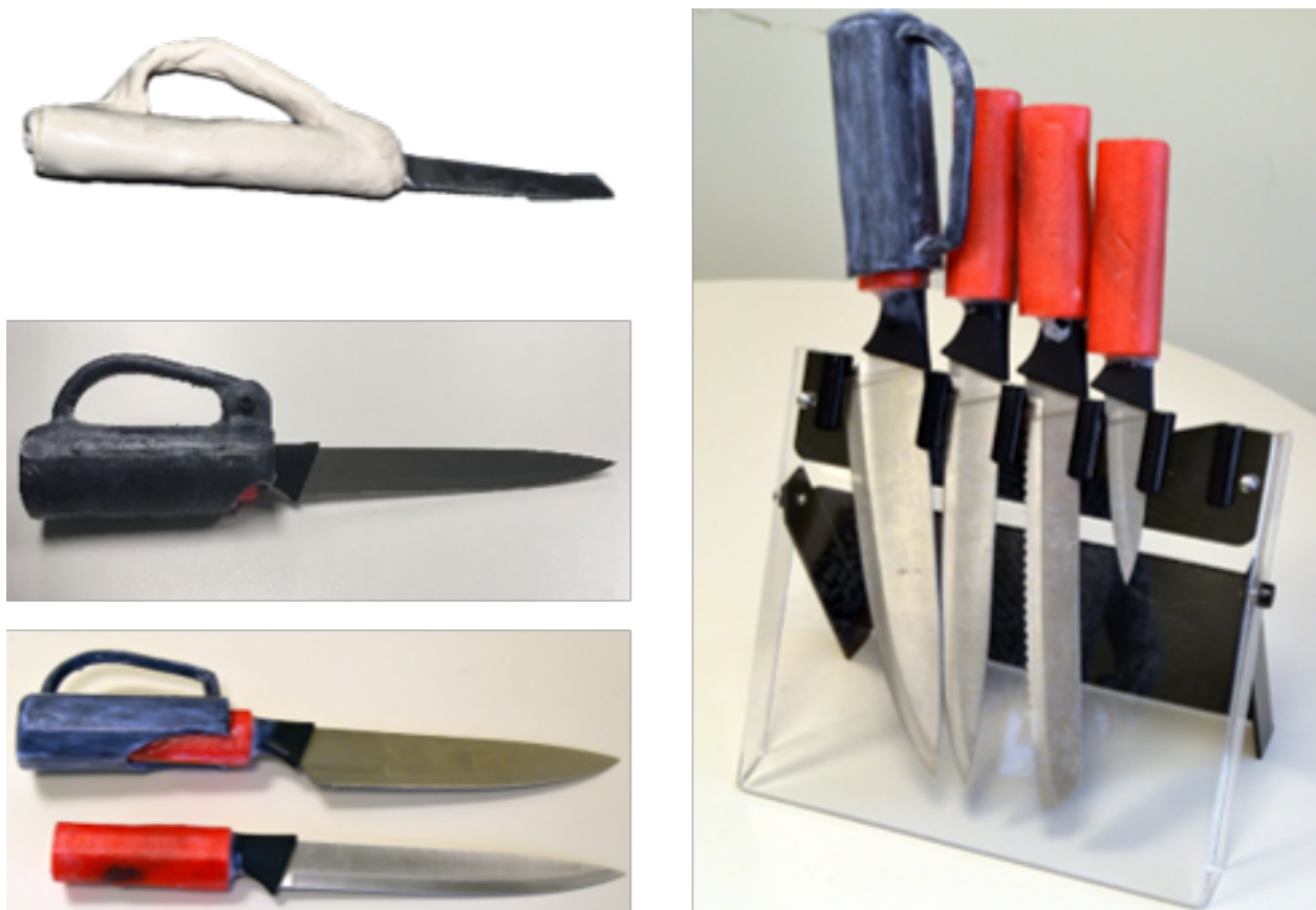
Figure 2: These images show the design progression of Jon's modular knife grip: Lorelai's original Orthoplast grip (top left); the initial pass at a 3D printed grip (middle left); a final design with red flexible inserts (bottom left, right)
