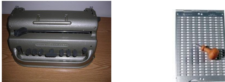
Figure 2: (a) [4] Brailier (b) [6] New slate and stylus allows users to read as they write
