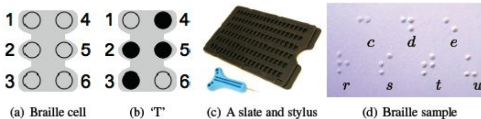
Figure 1[1]: (a) Schematic of a Braille cell (b) The Braille letter “T”: The black circles represent embossed dots, and the light grey circles represent the positions of the dots that are not embossed (c) A traditional slate and stylus (d) Written Braille
