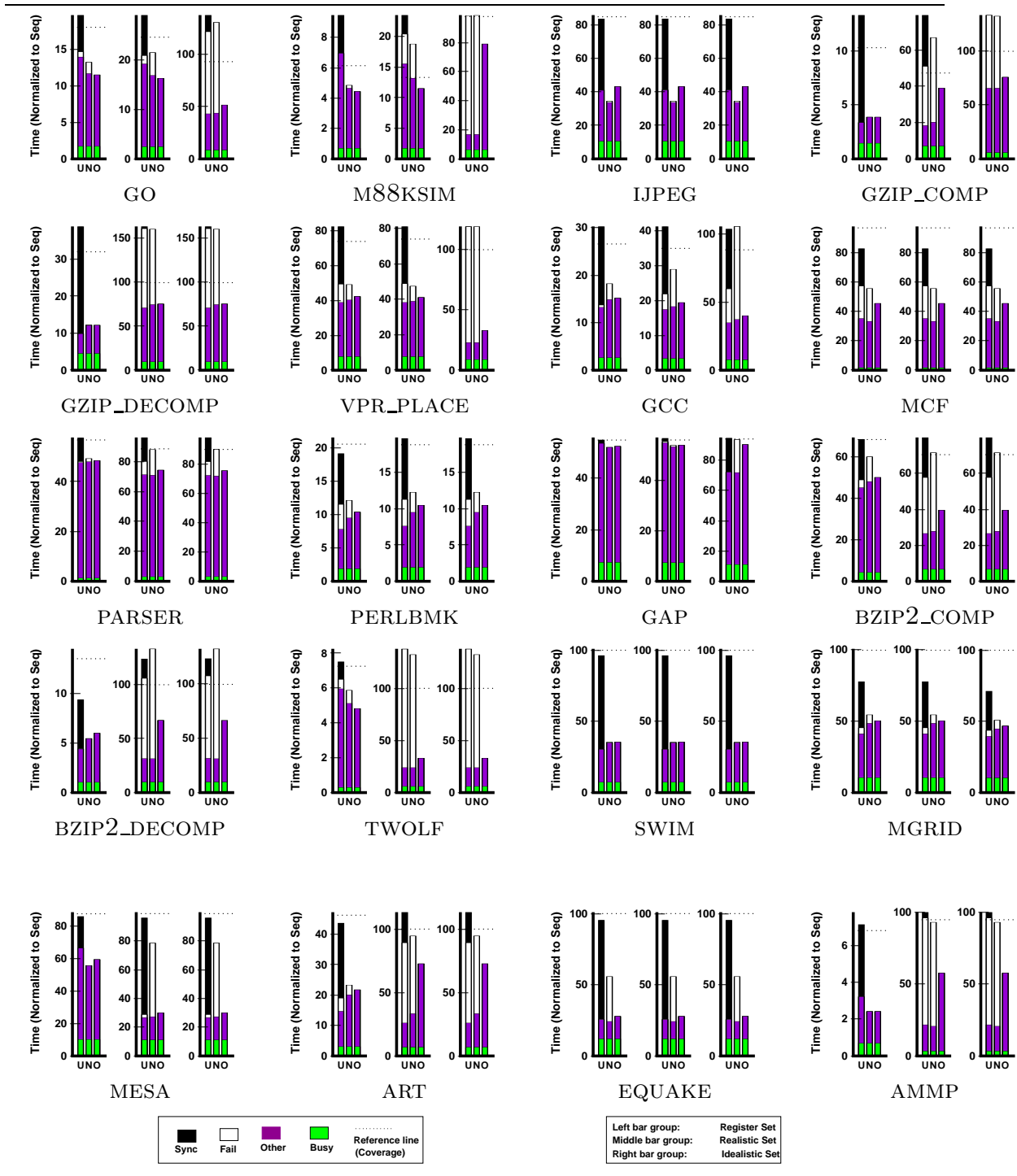
Figure 5.6: Potential impact of optimizing inter-thread value communication. For each benchmark, three sets of results are presented, corresponding to the register, the realistic, and the idealistic loop sets, respectively. Bars represent execution time of the parallel loops on a four-processor CMP normalized to the sequential program execution time. U is unoptimized, all register-resident values are synchronized and all memory-resident values are speculated; N assumes a perfect value predictor for all register-resident values; and O assumes a perfect value predictor for all values.
