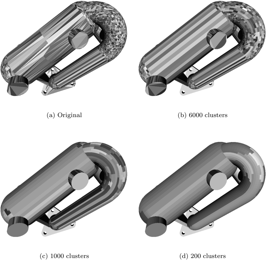
Figure 8.4: Sample clusters on the heat exchanger.
