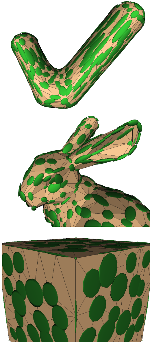
Figure 4.1: Quadric error isosurfaces on three simplified models: blobby “V”, bunny, and the corner of a cube. Note how the ellipsoids follow the local shape of each surface.
