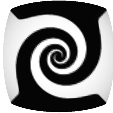
Figure 5.1: A section of a sphere Gouraud-shaded with a swirl pattern. Each vertex has a single associated color.
