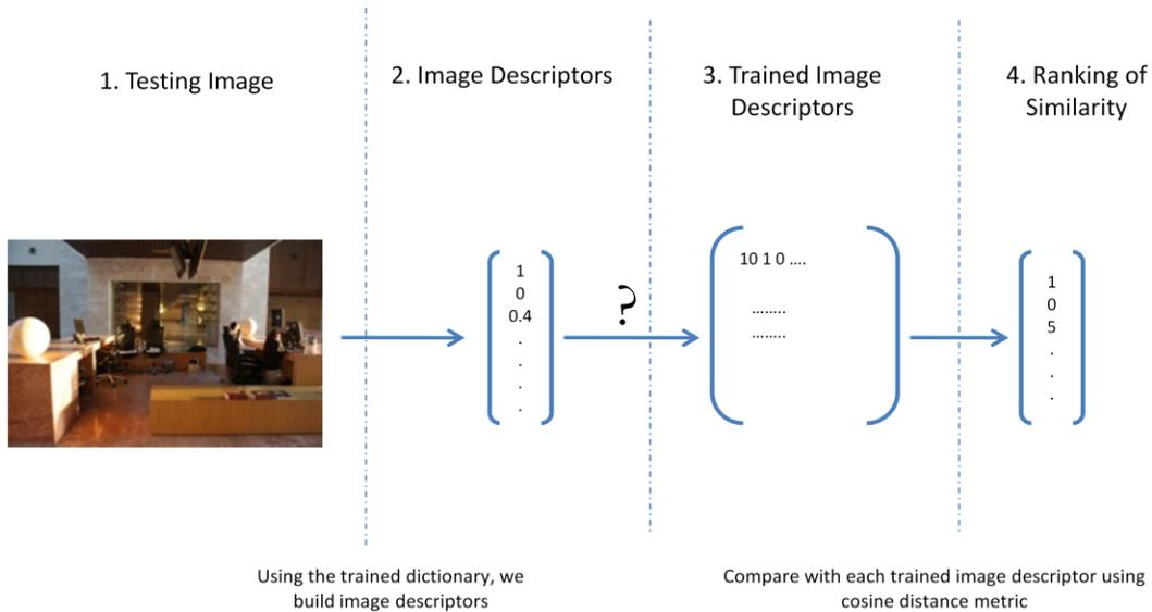
**Figure 6 Graphical Representation of the Basic Image Retrieval System**
