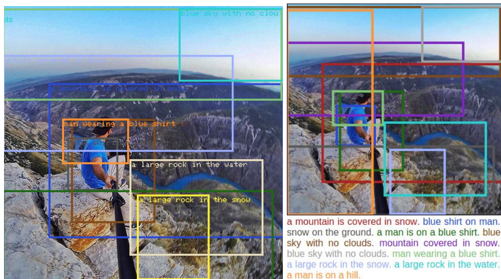
Figure 5.7: An example of the DenseCap on one of the images (Left) from our dataset. We use the dense captions produced by DenseCap (Right) to come up with text based features over them.
