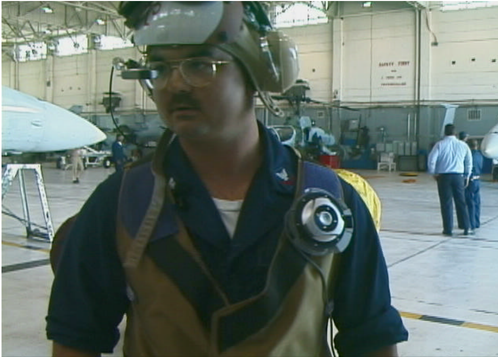
Figure 1: Maintainer wearing vest containing IBM wearable computer with dial for I/O and head-worn display on cranial cap in front of right eye
