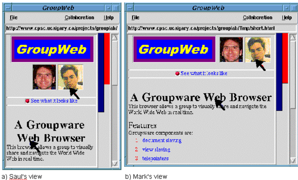
Figure 2. In a collaborative Web browser for use by multiple people, each person's telepointer must be placed in an appropriate place on everyone else's screen. This requires knowing where the individual words are since browsers reformat the text based on the current window width. (Figure reproduced from [5] with permission.)
