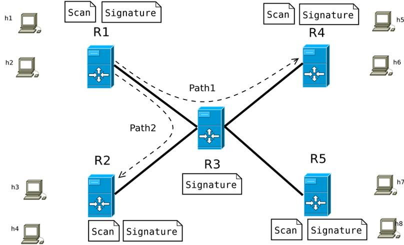
Figure 1: Example of network-wide NIDS instrumentation
