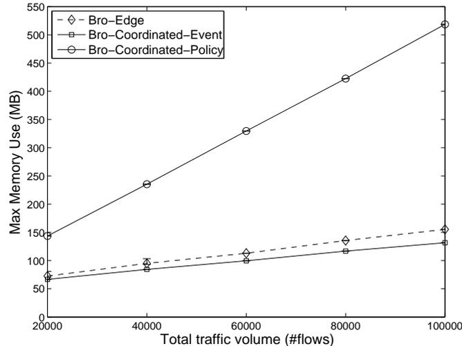
Figure 7: Max memory usage across the network as the total traffic volume increases
