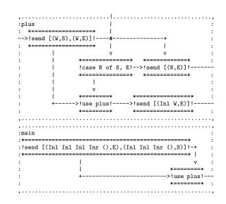
Figure 5: 2D program that adds the unary numbers 3 and 2.
