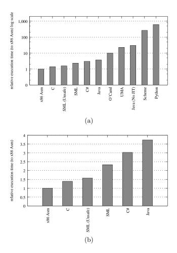
Figure 13: UM Performance. These graphs show the relative performance of different UM implementations. The top graph shows a large set of implementations on a logarithmic scale; the bottom graph shows only the best performing implementations on a linear scale. The judges admit that they are not experts in many of these languages and caution that these results should only be used to show that the UM can be implemented efficiently in several high-level languages.
