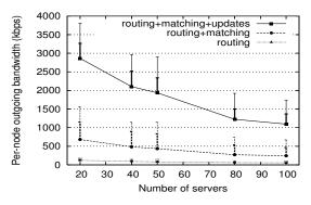
Figure 7: Scaling in per-node bandwidth consumption as the number of servers in the system increases when the number of players is fixed at 400.
