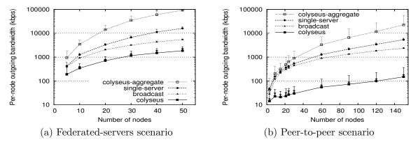
Figure 6: Scaling in per-node bandwidth usage as the number of servers in the system increase in (a) the federated-servers scenario and (b) the peer-to-peer scenario. (Note the logarithmic scale.)
