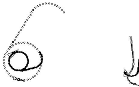
Figure 5.4. The first snapshot demonstrates the ability of the plane to survive indefinitely by flying in continuous circles within the missile's turn radius. The second snapshot demonstrates the learned behavior of the plane to turn toward the missile to increase the distance between the two in the long term, a tactic used by pilots.
