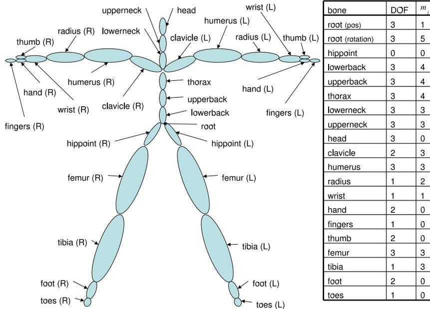
Figure 2: Human figure model, DOFs and the distribution of  $m_j$ . It has 29 joints, 56 joint angles, three angles for the root orientation and three position coordinates for the root.
