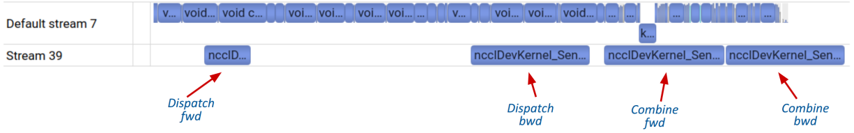
Figure 4.1: Nsight Systems trace of a Qwen3-235B-A22B training step. Compute kernels run on the default CUDA stream (top); dispatch and combine all-to-all kernels run on a separate NCCL stream (bottom).
