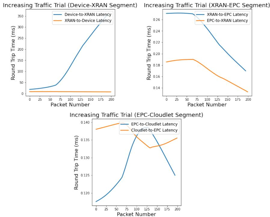
**Figure 11: Segment Latencies Observed for Increasing Traffic Trial**
