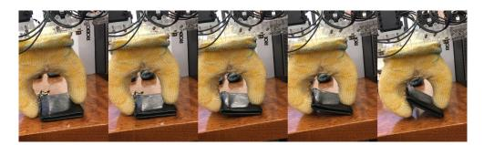
Figure 8.8: Hardware results for motion 1. Screenshot 1: initial position. Screenshots 2-3: motion with front fingers. Screenshots 4-5: motion with back fingers.
