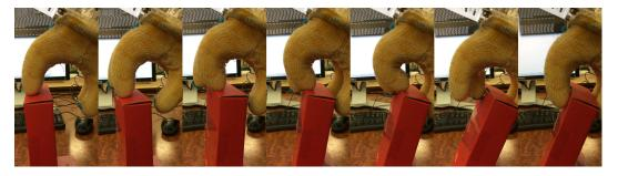
**Figure 8.10:** Hardware results for motion 3. Screenshots 1-3: initial position and motion with front fingers. Screenshots 4-5: motion with back fingers. Screenshots 6-7: front finger reset and first frame of motion.
