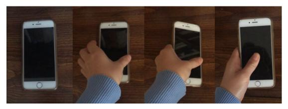
Figure 8.1: When a phone is lying flat on a table, its bottom surface is blocked (far left). However, contacts with this bottom surface are needed in the desired grasp (far right). To achieve this grasp, intermediate levering up is performed.
