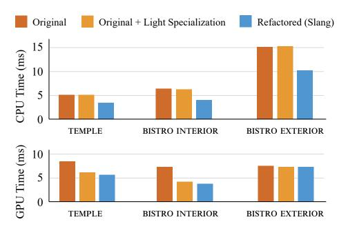
Figure 5.4: Comparing average per-frame CPU time (top) and GPU time (bottom) of the original branches (with and without light specialization), and the refactored branch of the Falcor renderer, we find that the refactored renderer improves CPU performance and preserves the same level of GPU performance as the original branch with light specialization.
