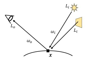
Figure 2.4: Explanation of rendering equation.  $L_o$  is the amount of light (radiance) reflected by the surface point into the camera.  $\omega_o$  is the view direction,  $\boldsymbol{x}$  is the location of the surface point where appearance is being computed.  $\omega_i$  represents an incoming light direction,  $L_i(\boldsymbol{x}, \omega_i)$  is the incoming radiance along direction  $\omega_i$ , and  $\boldsymbol{n}$  is the normal vector of the surface. f is a BxDF.
