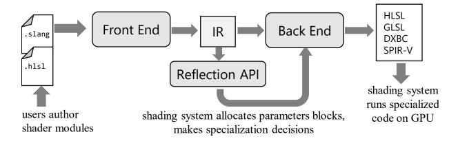
Figure 4.1: The Slang system implementation comprises a compiler front-end (for checking and determining parameter layouts for unspecialized modules) and back-end (for generating specialized GPU kernels), as well as supporting APIs. Applications use the Slang reflection API to obtain shader parameter layout information used to allocate GPU parameter blocks and to guide the specialization choices needed for low-level code generation.
