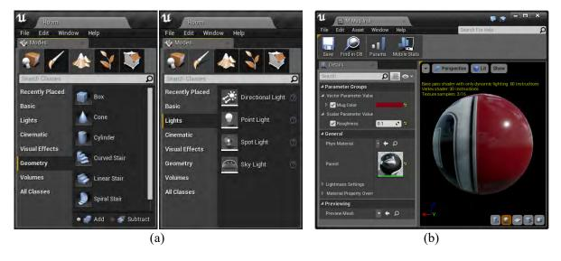
Figure 2.2: The GUI tools in Unreal Engine 4 reflects a typical graphics engineer's mental decomposition for the shading problem. (a) Partial screenshots of Unreal Engine 4's level editor show different types of geometry and lights. (b) Unreal Engine 4's material editor allows a user to define object's visual appearances.
